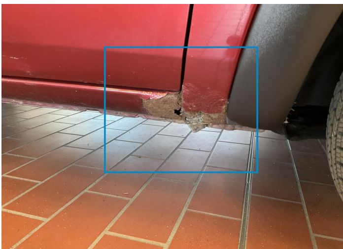
8. Rocker Panel / Center Right Paint / Corrosion -
