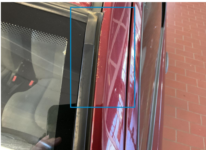
10. Pillar / Front Left Paint / Corrosion -
