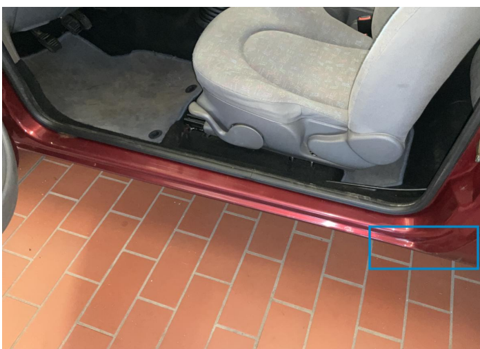
16. Rocker Panel / Center Left Paint / Corrosion -
