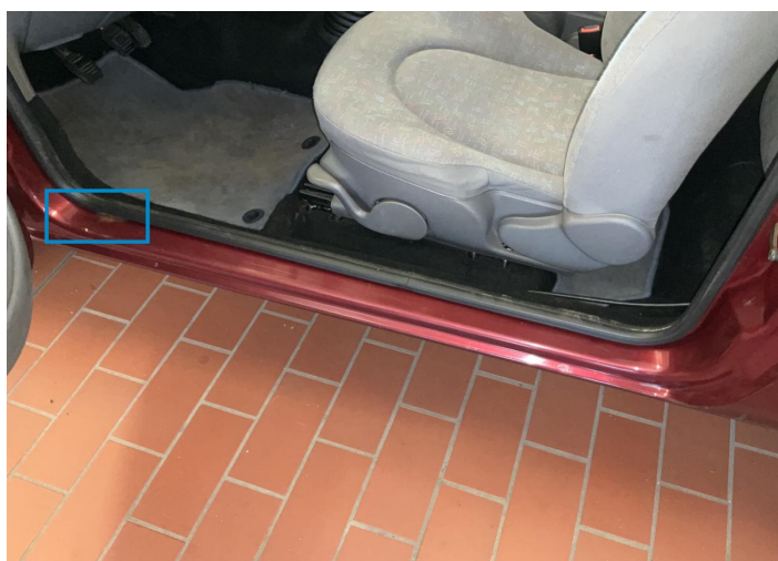
15. Rocker Panel / Center Left Paint / Corrosion -
