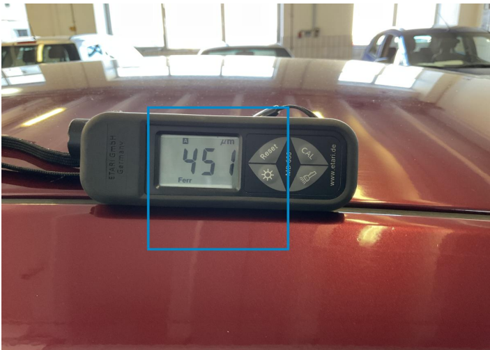
2. Roof Paint / Poor Previous Repair -
