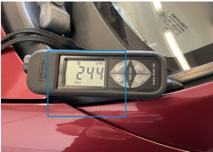
1. Door / Front Left Paint / Poor Previous Repair -
