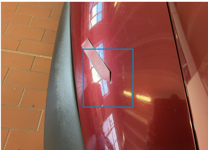
12. Fender / Front Right Paint / Chipping -
