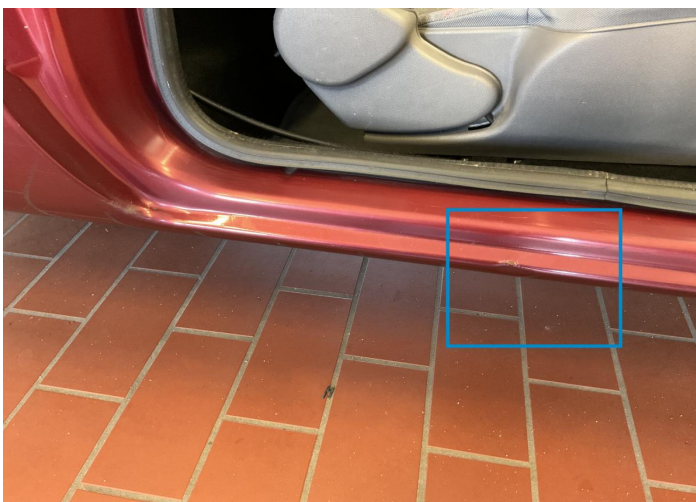
14. Rocker Panel / Center Right Paint / Corrosion -
