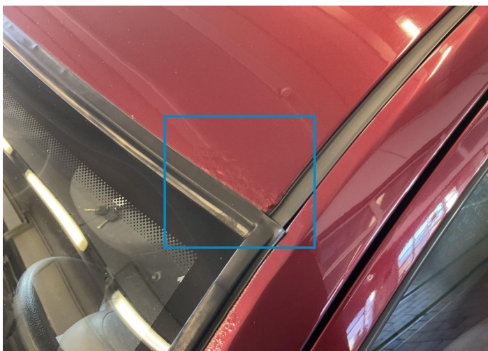
11. Roof Paint / Corrosion -
