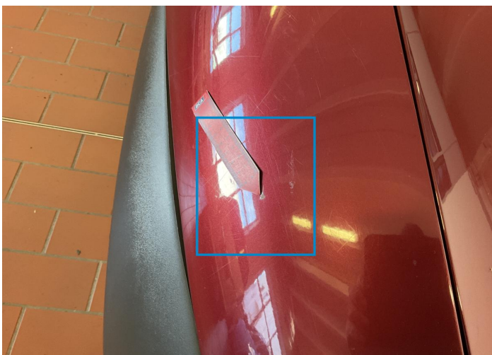
12. Fender / Front Right Paint / Chipping -
