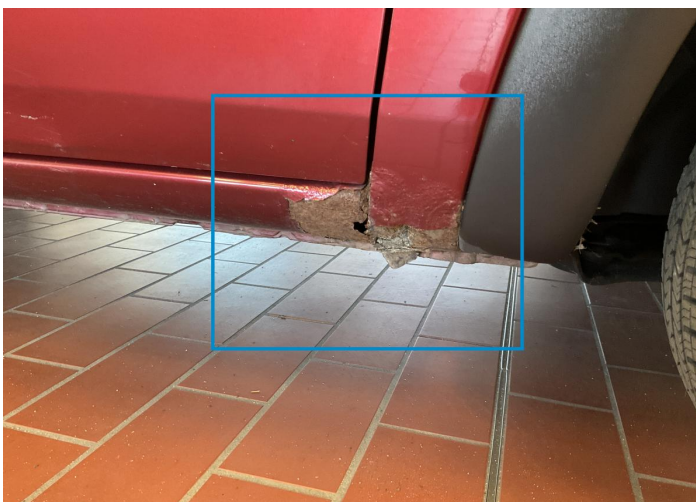
8. Rocker Panel / Center Right Paint / Corrosion -
