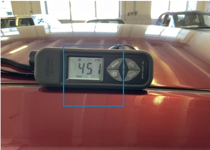
2. Roof Paint / Poor Previous Repair -
