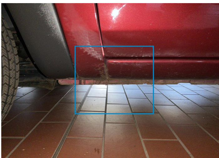
9. Rocker Panel / Center Left Paint / Corrosion -
