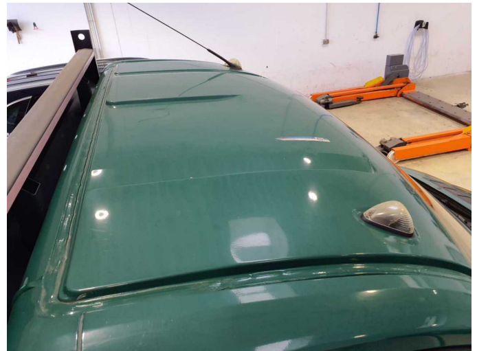
Damage 15: Roof: Roof - Deformed - Repair and paint
