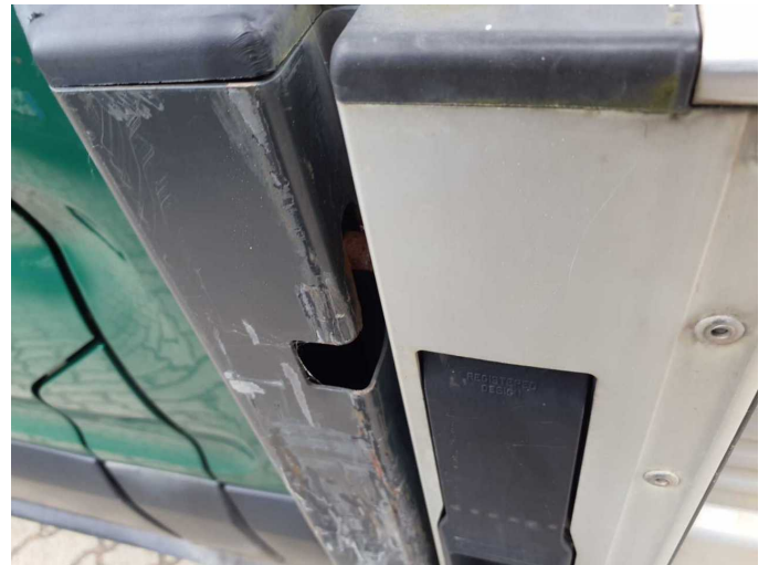
Damage 6: Trim / covers: Cargo area - lining -left side (Außen) - Loose - Un- / install
