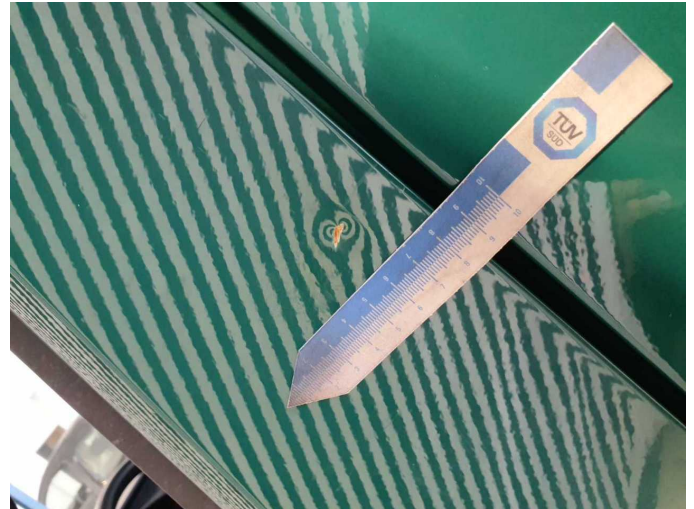
Damage 13: Door - front left side: Door - Corrosion - Repair and paint
