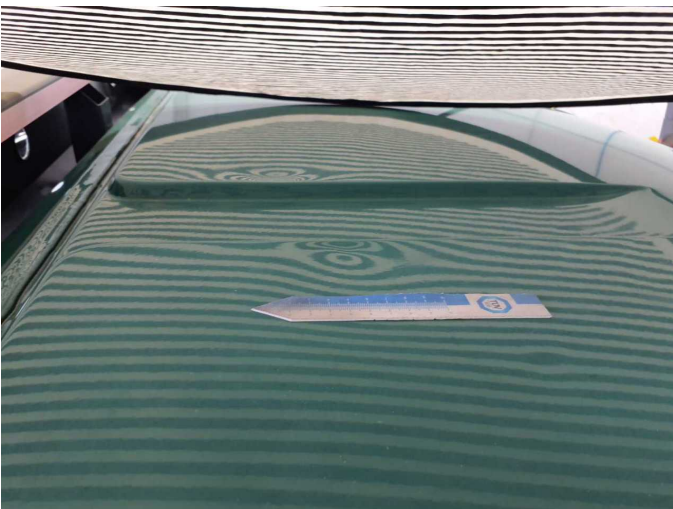
Damage 15: Roof: Roof - Deformed - Repair and paint
