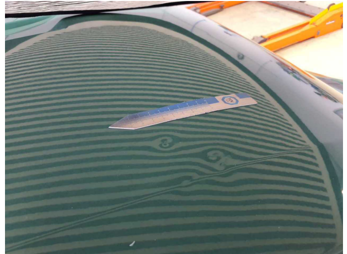
Damage 15: Roof: Roof - Deformed - Repair and paint
