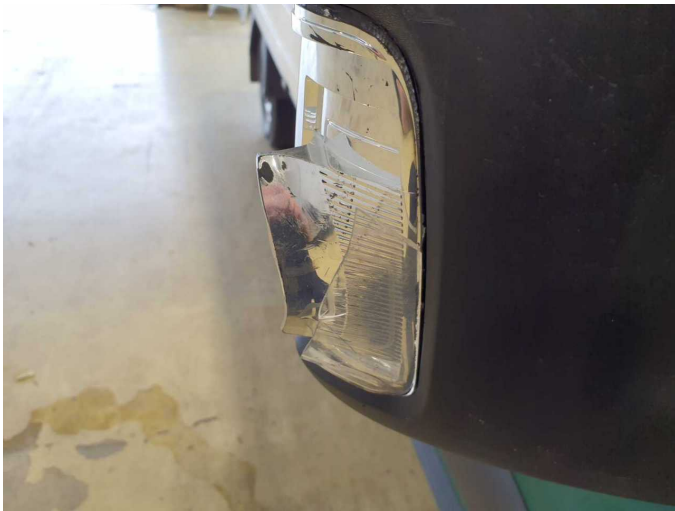
Damage 8: Indicator - front: Mirror - right side - Damaged - Replace
