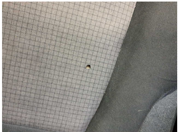
Damage 12: Seat - front: Seat cover - right side - Burn hole (cigarettes) - Replace
