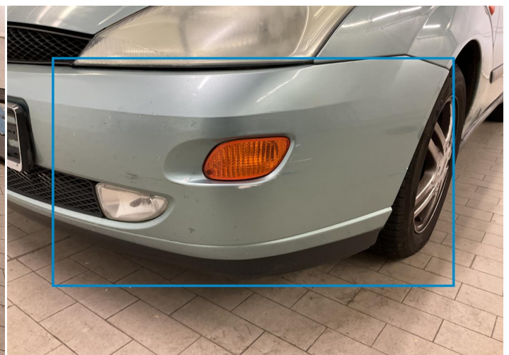
6. Bumper / Front Paint / Scratch / Scuff -
