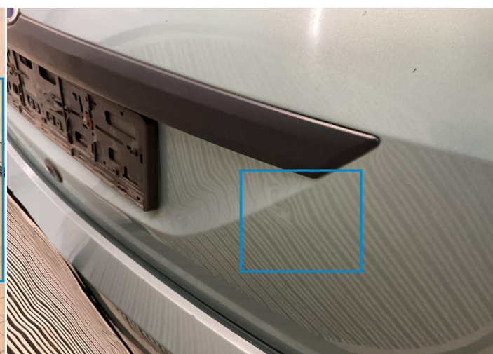
12. Tailgate light Bodywork / Dent / Dent -
