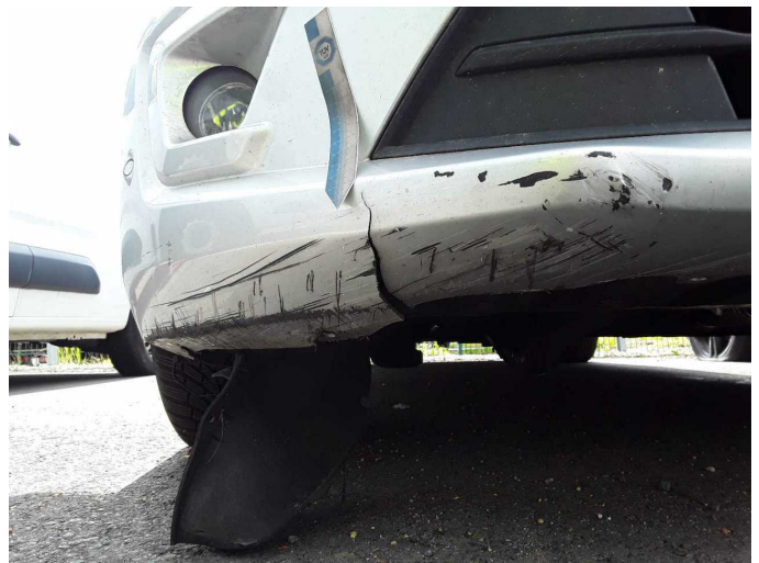
Damage 6: Front bumper: Front bumper - Damaged - Replace
