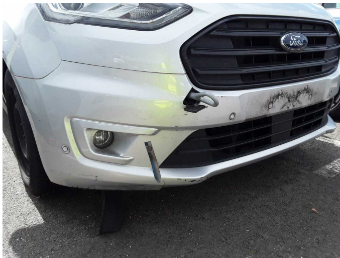
Damage 6: Front bumper: Front bumper - Damaged - Replace
