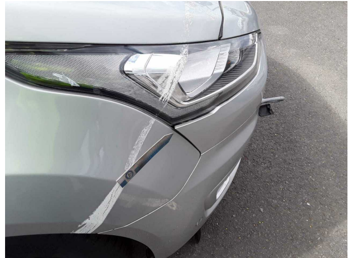
Damage 6: Front bumper: Front bumper - Damaged - Replace
