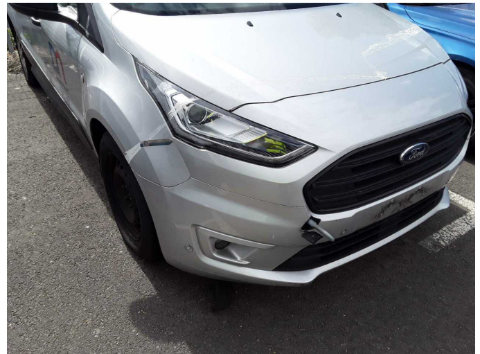
Damage 6: Front bumper: Front bumper - Damaged - Replace
