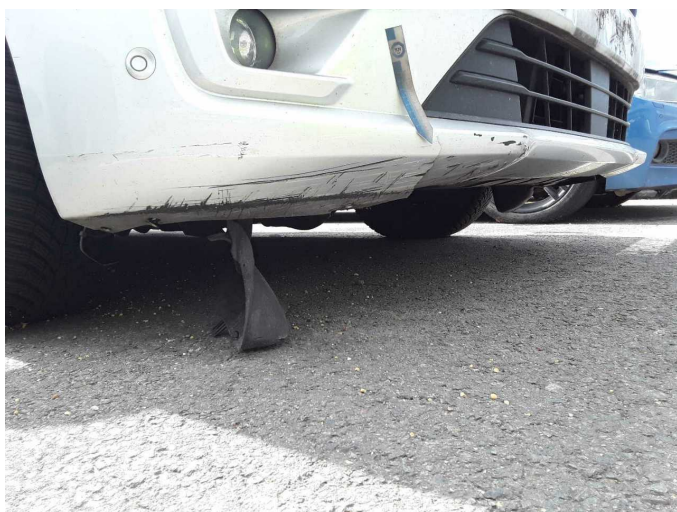
Damage 6: Front bumper: Front bumper - Damaged - Replace
