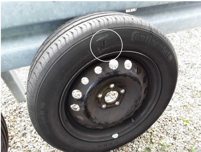
Damage 2: 2nd wheel set: 1 tyre - Broken / torn - Replace
