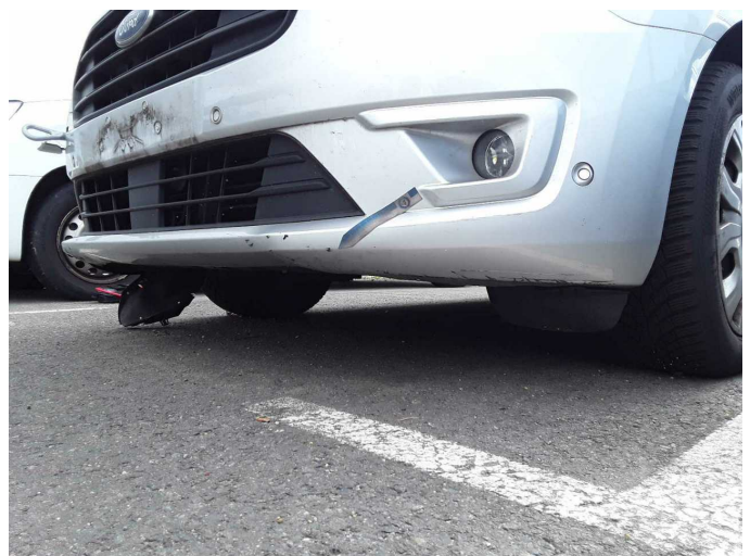
Damage 6: Front bumper: Front bumper - Damaged - Replace
