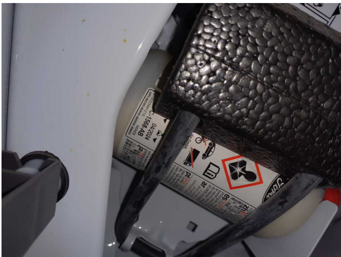
Damage 1: Equipment: Tirefit filler - Expired - Replace
