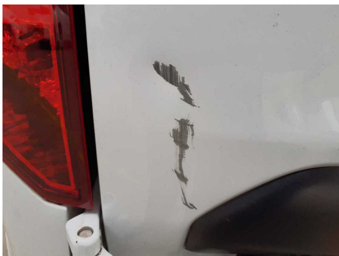
Damage 4: Boot lid / rear door: Rear door - left side - Scratched - Paint
