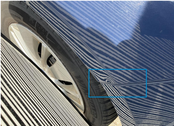
3. Fender / Front Right Bodywork / Dent / Dent -
