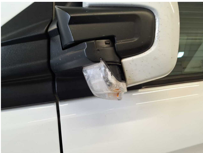
Damage 2: Indicator - front: Mirror - left side - Soiled - Replace
