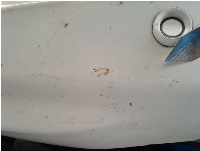
Damage 12: Front bumper: Bumper with Parktronic (Unterteil) - Deformed - Replace
