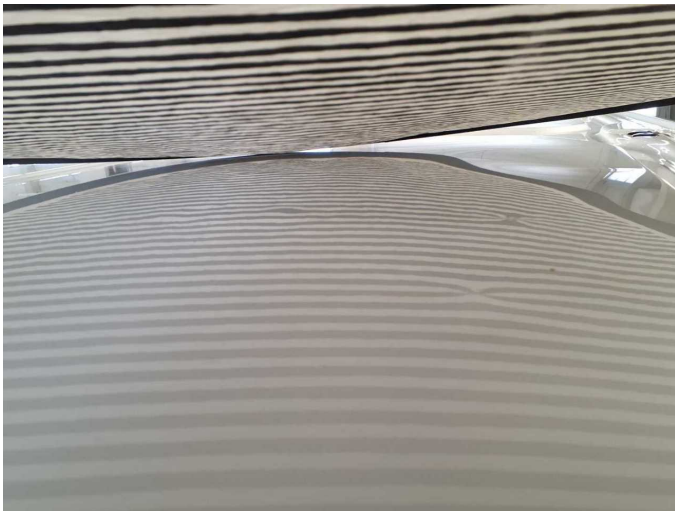
Damage 16: Roof: Roof - dent(s) - Repair and paint
