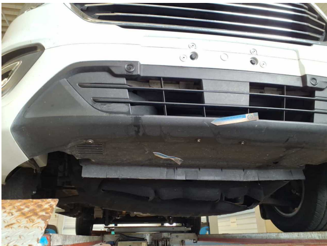
Damage 5: Front bumper: Air-inlet grille - Scratched - Replace
