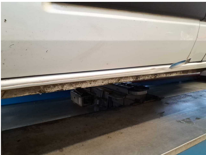
Damage 13: Sill - left side: Sill - dent(s) - Repair and paint
