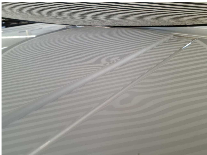
Damage 16: Roof: Roof - dent(s) - Repair and paint
