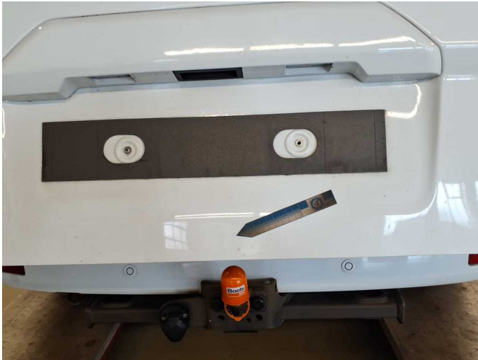
Damage 3: Boot lid / rear door: Boot lid glazed - dent(s) - Smart repair
