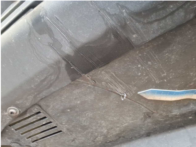
Damage 5: Front bumper: Air-inlet grille - Scratched - Replace
