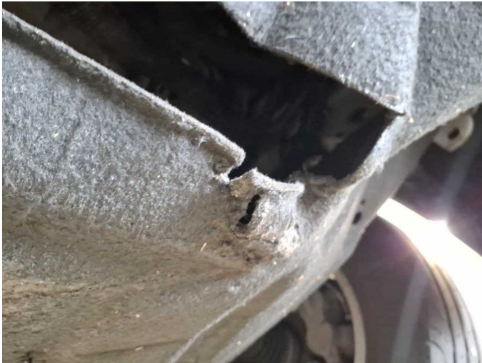
Damage 9: Engine: Engine cowling lower front - Broken / torn - Replace
