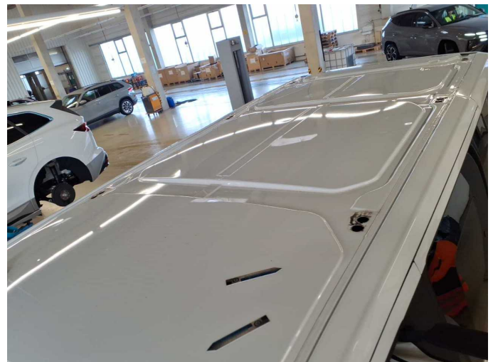
Damage 16: Roof: Roof - dent(s) - Repair and paint
