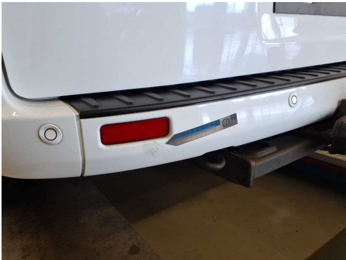
Damage 4: Rear bumper: Bumper with Parktronic - Unprofessionally repaired - Smart repair
