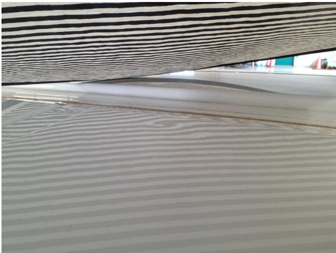
Damage 16: Roof: Roof - dent(s) - Repair and paint
