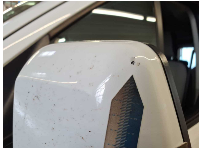
Damage 1: Wing mirror - left side: Cap - Scratch(es) - Paint
