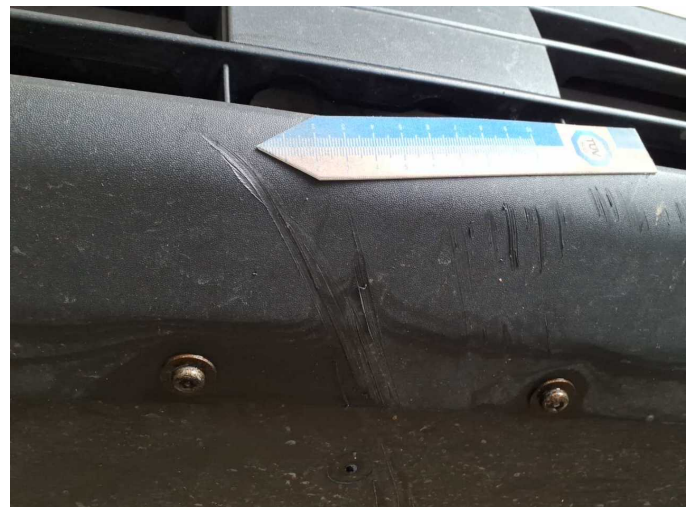
Damage 5: Front bumper: Air-inlet grille - Scratched - Replace
