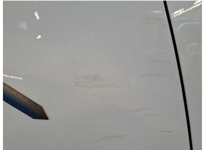
Damage 15: Side panel - rear right side: Side panel - Deformed - Repair and paint
