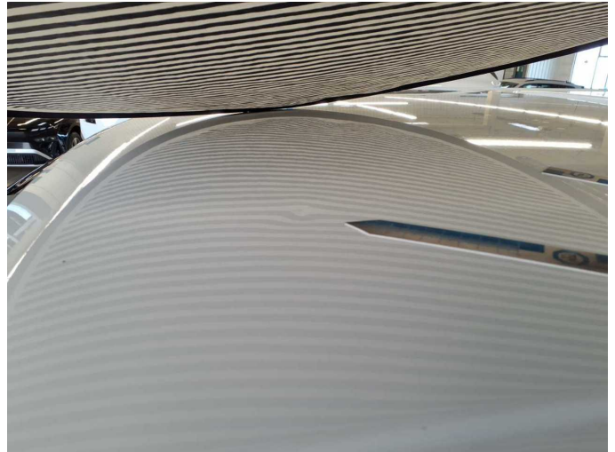
Damage 16: Roof: Roof - dent(s) - Repair and paint
