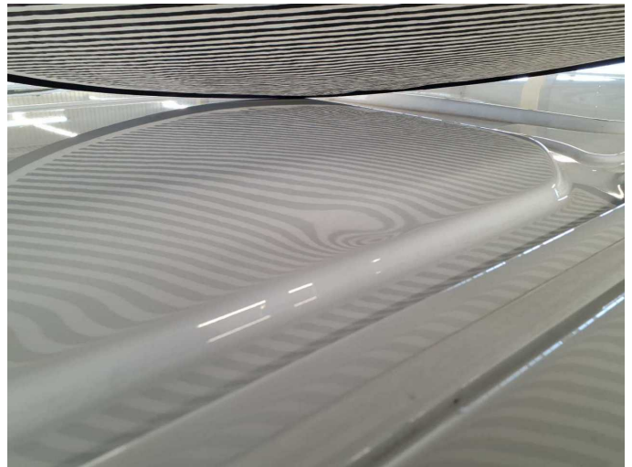
Damage 16: Roof: Roof - dent(s) - Repair and paint
