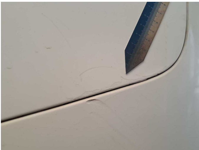
Damage 11: Side panel - rear left side: Side panel - Unprofessionally repaired - Paint
