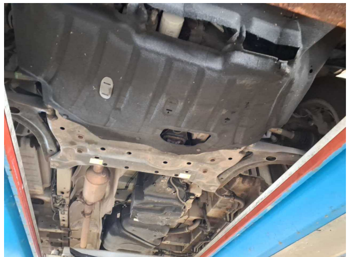
Damage 9: Engine: Engine cowl lower front - Broken / torn - Replace
