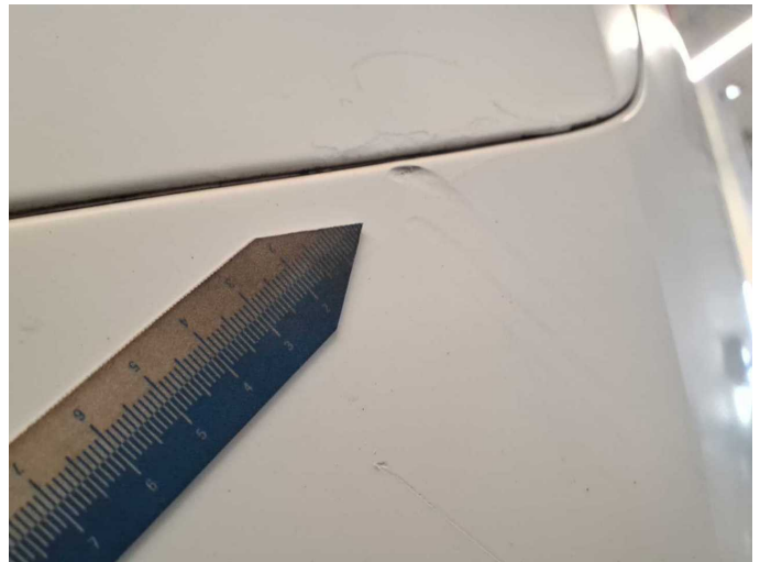
Damage 6: Rear bumper: Bumper - rear left side - Deformed - Replace
