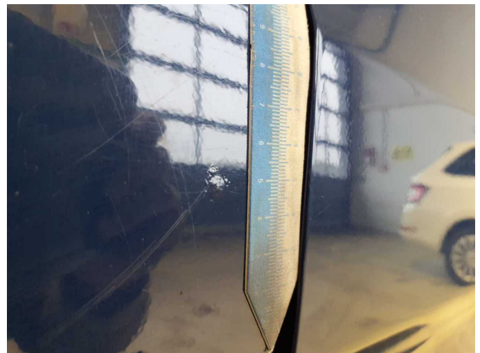
Damage 3: Boot lid / rear door: Rear door - left side - Corrosion - Repair and paint
