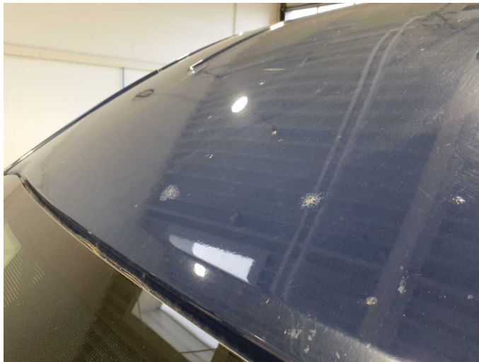
Damage 7: Roof: Roof - Corrosion - Repair and paint
