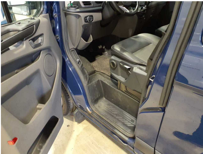
Damage 2: Sill - left side: Sill - Corrosion - Paint
