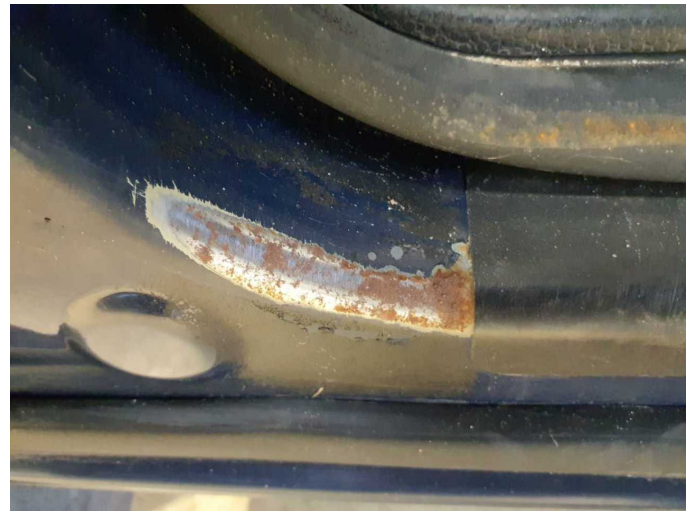
Damage 2: Sill - left side: Sill - Corrosion - Paint
