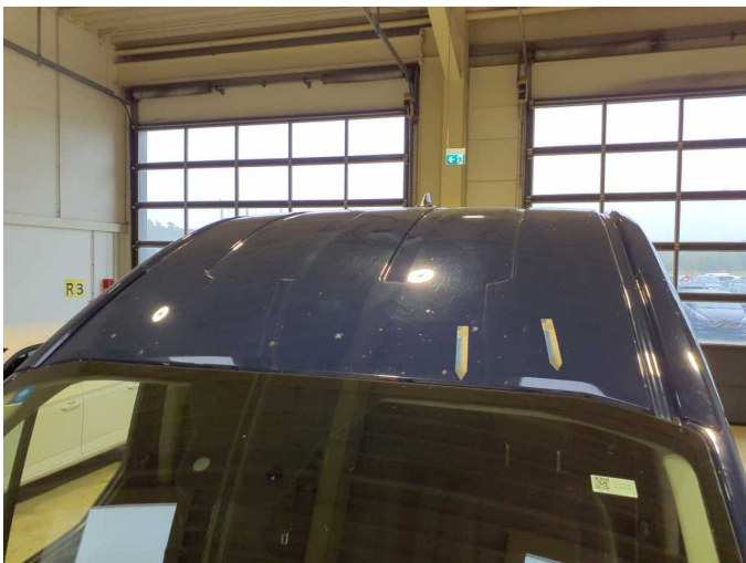
Damage 7: Roof: Roof - Corrosion - Repair and paint
