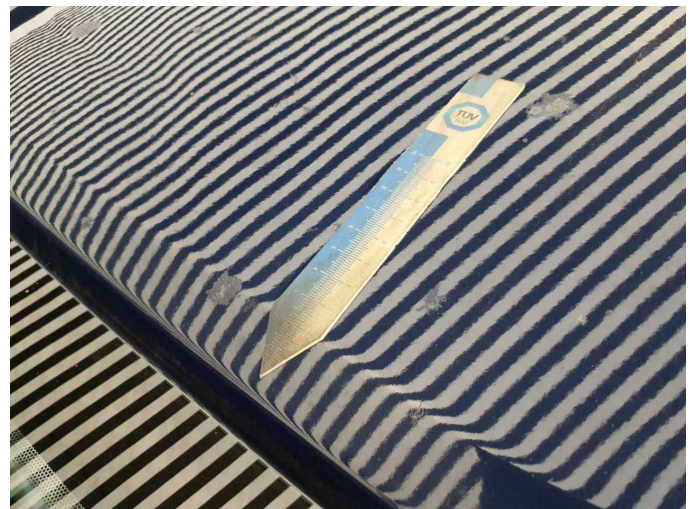
Damage 7: Roof: Roof - Corrosion - Repair and paint
