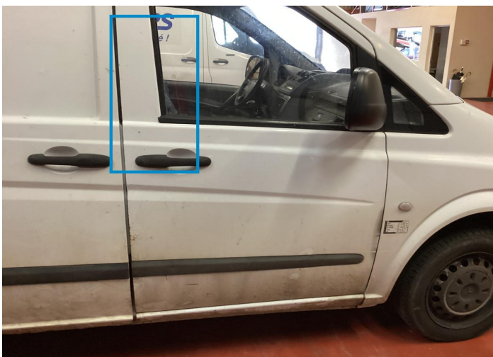
32. Door / Front Right Paint / Chipping -
