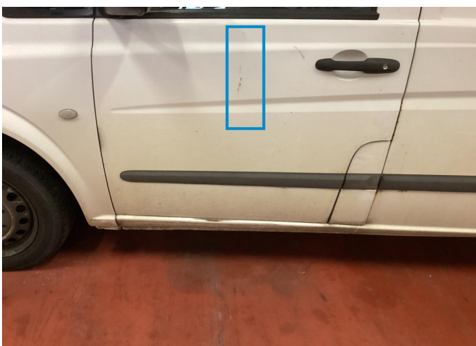
10. Door / Front Left Bodywork / Poor Previous Repair -
