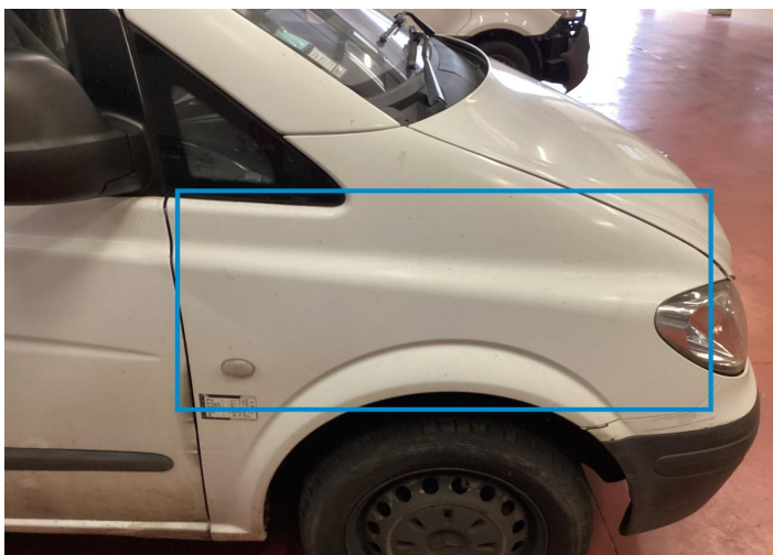
35. Fender / Front Right Paint / Chipping -
