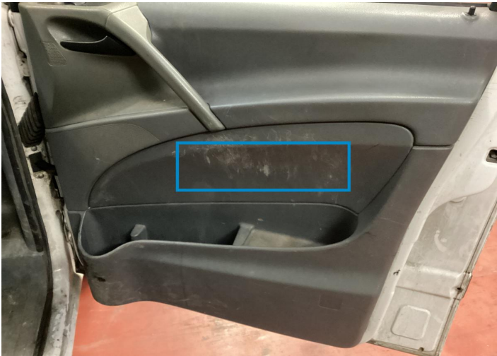
4. Panel Filling / Front Right Interior / Scraped -
