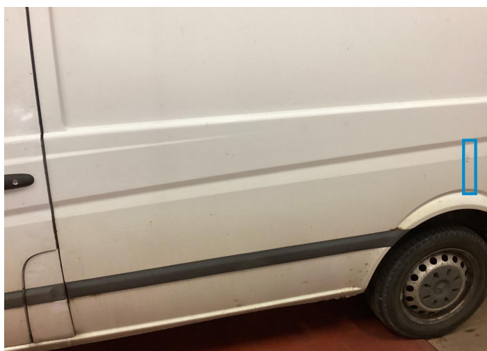
15. Fender / Back Left Bodywork / Poor Previous Repair -
