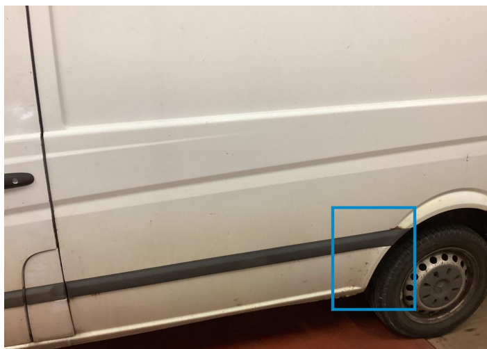
13. Fender / Back Left Paint / Corrosion -
