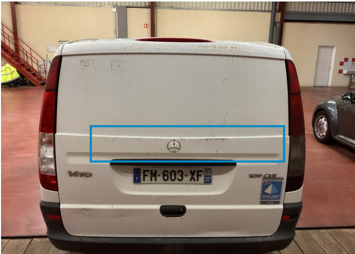
20. Tailgate Paint / Poor Previous Repair -
