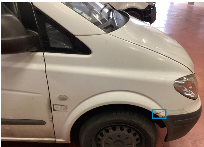
36. Fender / Front Right Bodywork / Breakage -
