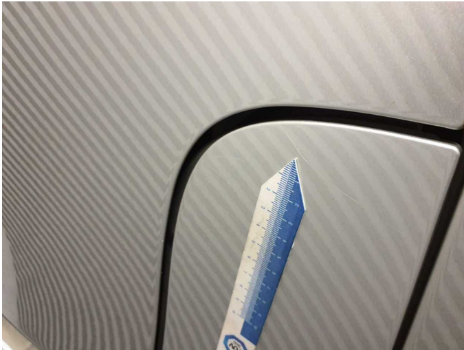
Damage 3: Fuel system: Tank cap - Scratched - Smart repair
