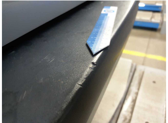
Damage 12: Rear bumper: Rear bumper - Scratched - Replace
