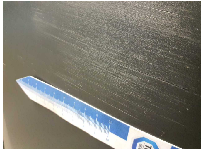
Damage 10: Front bumper: Front bumper - Scratched - Replace
