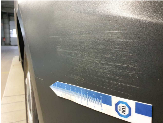
Damage 10: Front bumper: Front bumper - Scratched - Replace
