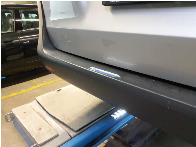
Damage 12: Rear bumper: Rear bumper - Scratched - Replace
