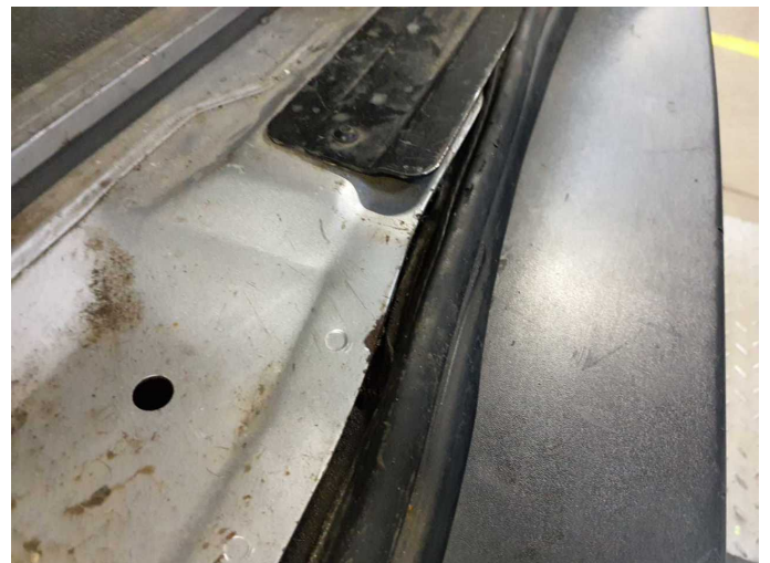
Damage 4: Boot lid / rear door: Seal - Malposition - Repair
