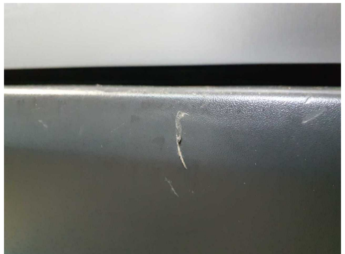
Damage 12: Rear bumper: Rear bumper - Scratched - Replace
