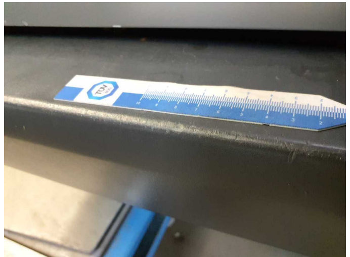
Damage 12: Rear bumper: Rear bumper - Scratched - Replace
