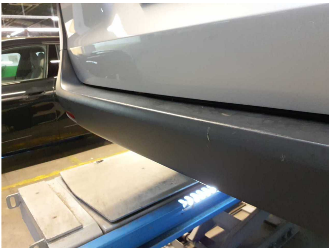
Damage 12: Rear bumper: Rear bumper - Scratched - Replace
