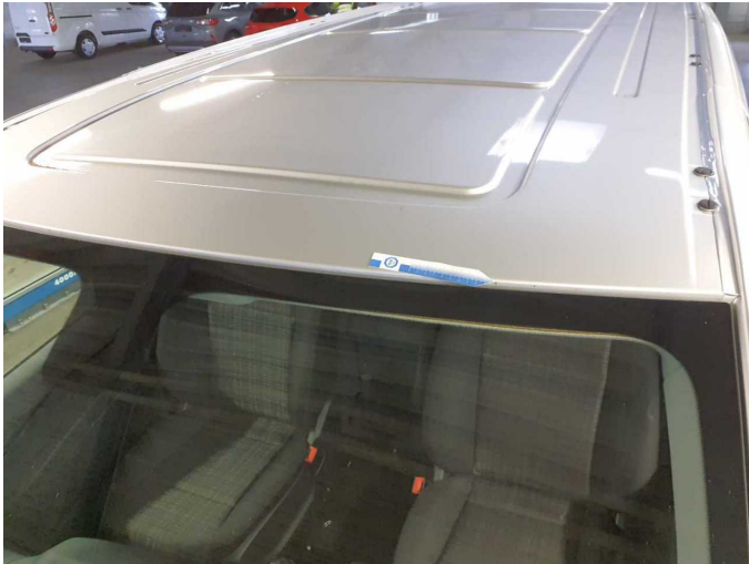
Damage 7: Roof: Roof - Corrosion - Smart repair
