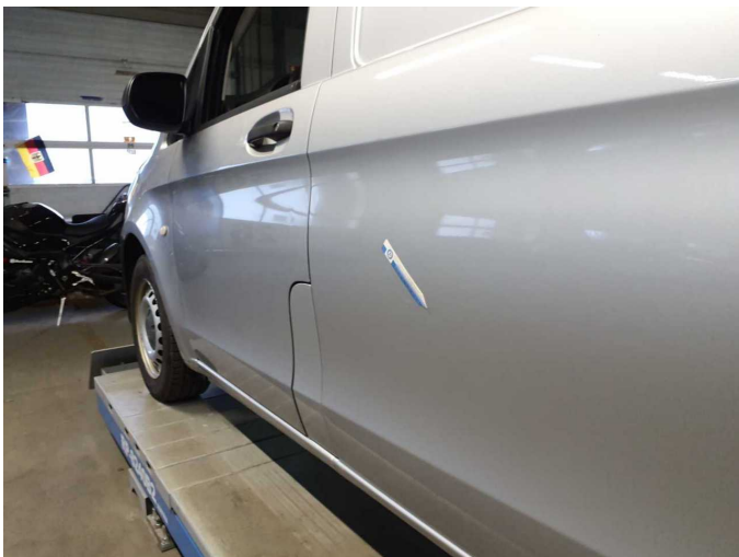
Damage 6: Side panel - rear left side: Side panel - Scratched - Smart repair
