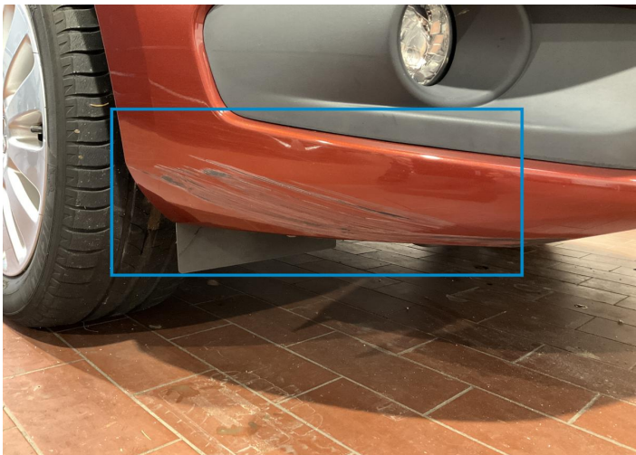
2. Corner Bumper / Front Right Paint / Scratch / Scuff -
