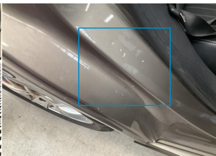
18. Pillar / Back Right Bodywork / Dent / Dent -
