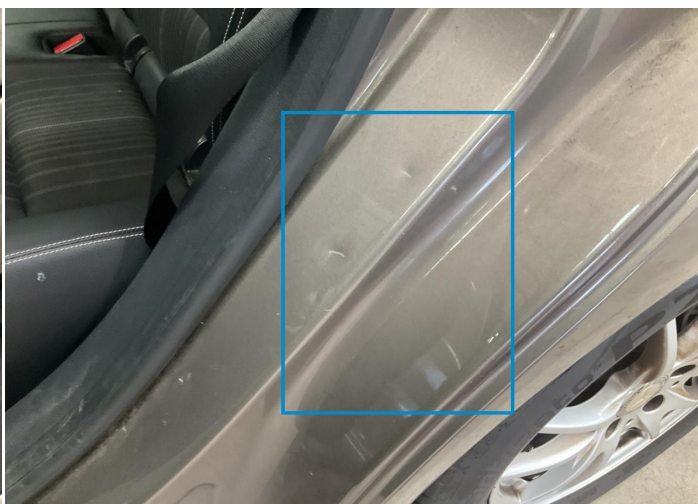
12. Pillar / Back Left Bodywork / Dent / Dent -
