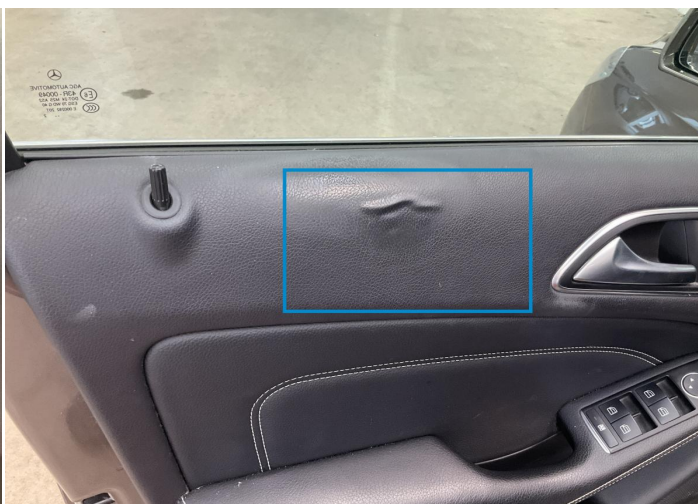
8. Panel Filling / Front Left Interior / Dented -
