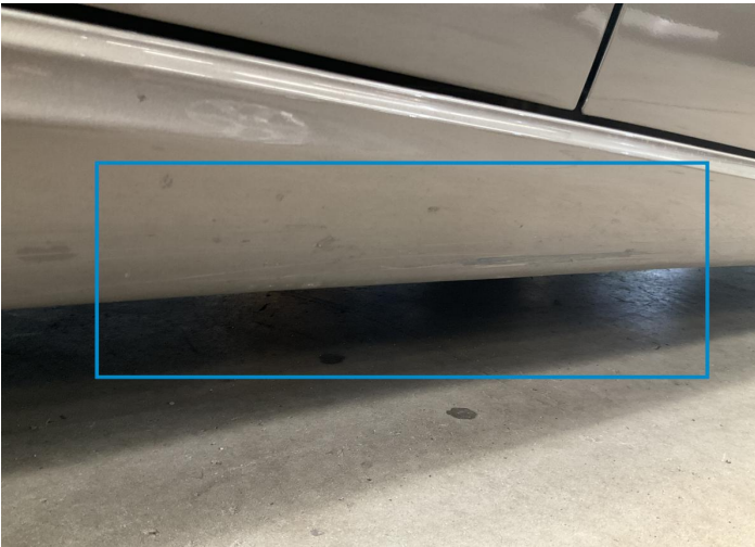
19. Rocker Panel / Center Right Paint / Scratch / Scuff -
