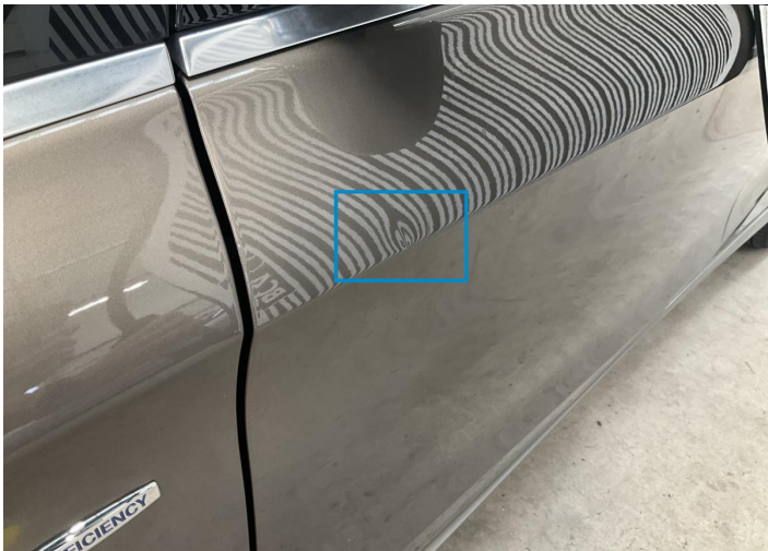
5. Door / Front Left Bodywork / Dent / Dent -
