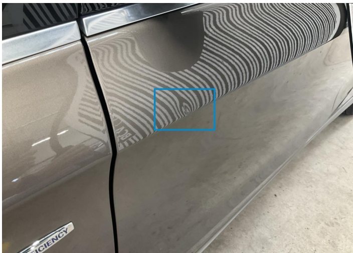
5. Door / Front Left Bodywork / Dent / Dent -
