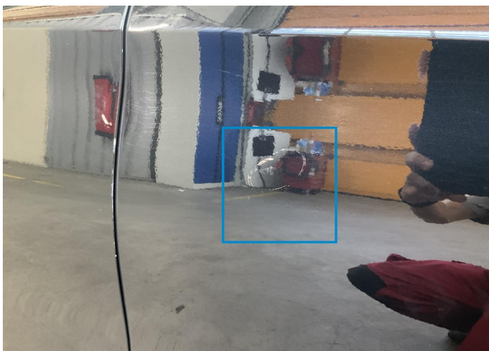
7. Door / Back Left Paint / Poor Previous Repair -
