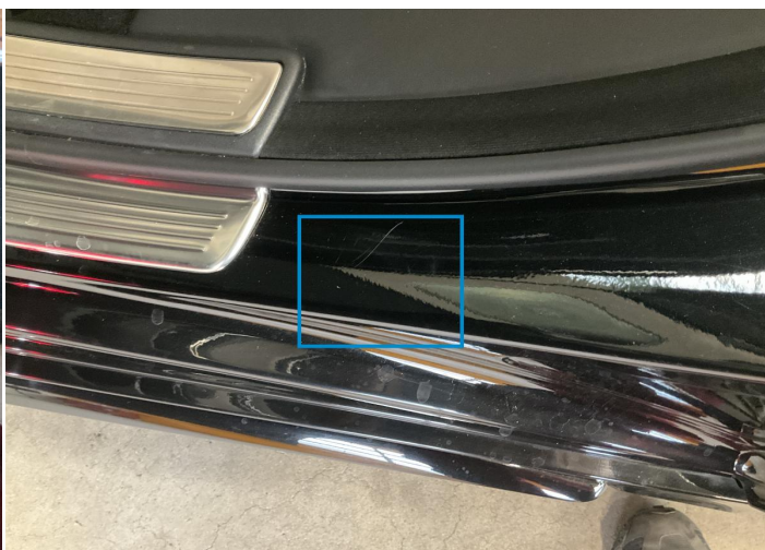
8. Pillar / Back Left Paint / Scratch / Scuff -
