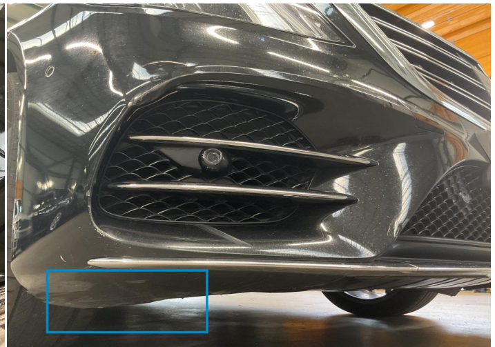
2. Bumper / Front Paint / Scratch / Scuff -
