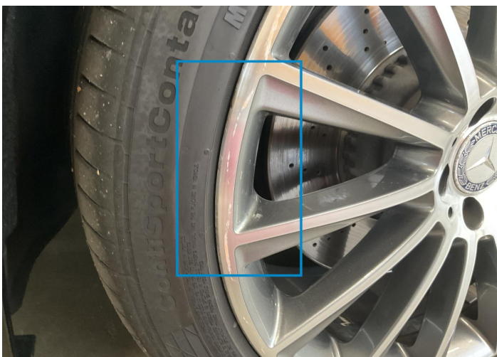
5. Rim / Front Left Out of Bodywork / Scratch -
