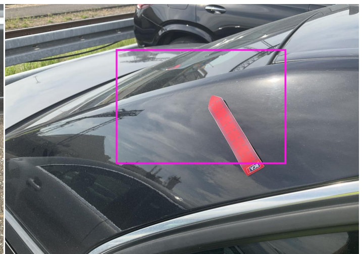
12. Roof Paint / Scratch / Scuff -
