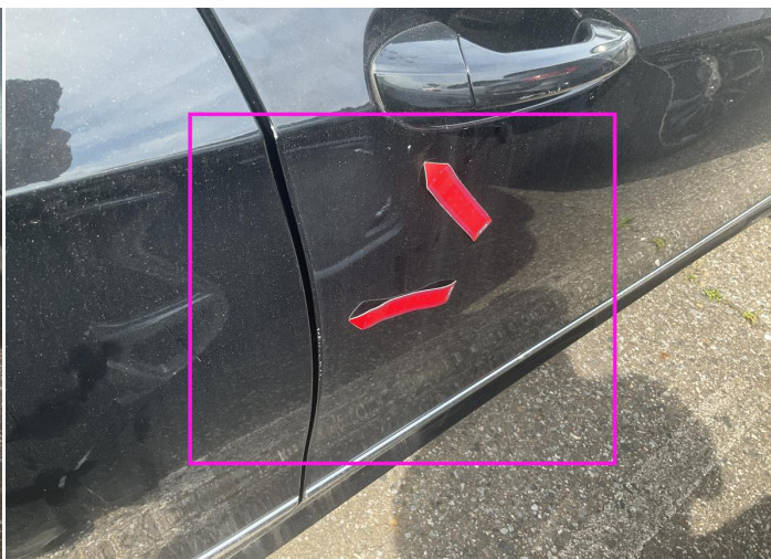
16. Door / Front Right Paint / Scratch / Scuff -
