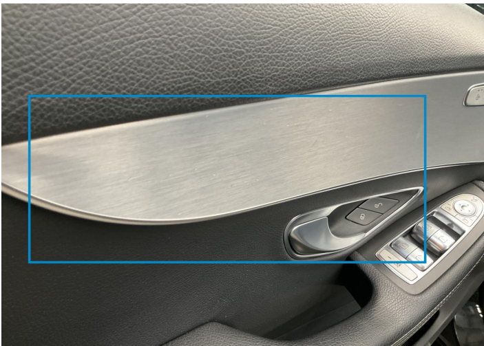
2. Panel Filling / Front Left Interior / Scratched -
