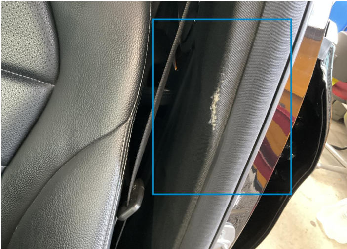
3. Door Step / Front Left Interior / Distorted -
