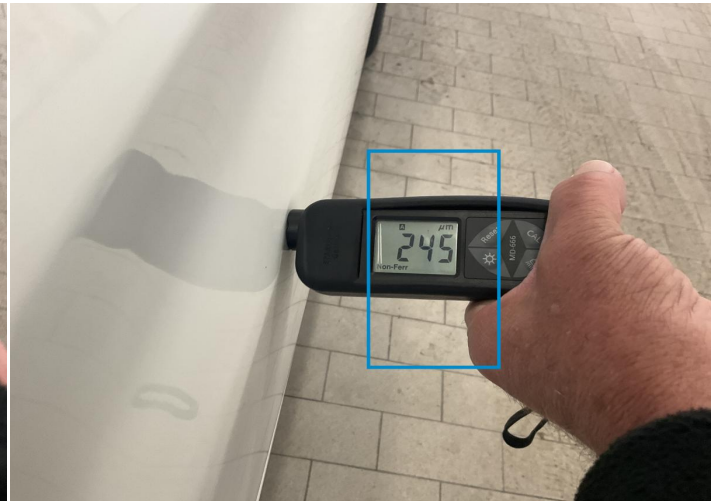
14. Door / Front Right Paint / Poor Previous Repair -
