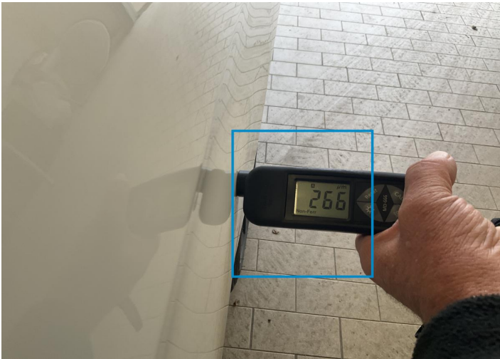
10. Door / Back Left Paint / Poor Previous Repair -
