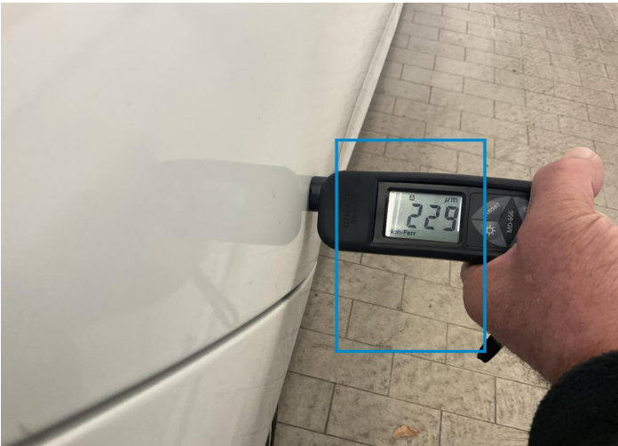
15. Door / Back Right Paint / Poor Previous Repair -
