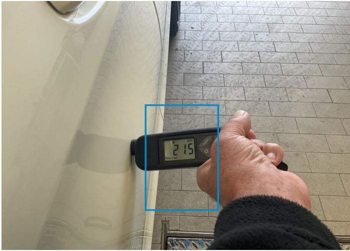
11. Door / Front Left Paint / Poor Previous Repair -
