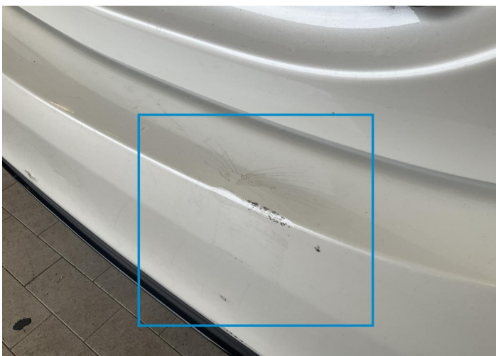
17. Bumper / Back Bodywork / Breakage / Crack -
