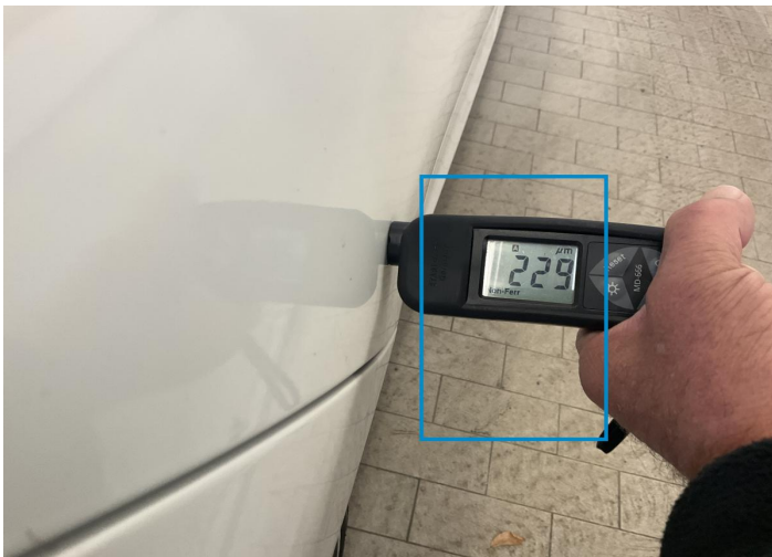
15. Door / Back Right Paint / Poor Previous Repair -
