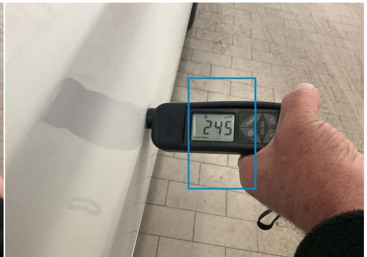
14. Door / Front Right Paint / Poor Previous Repair -
