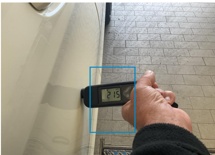
11. Door / Front Left Paint / Poor Previous Repair -
