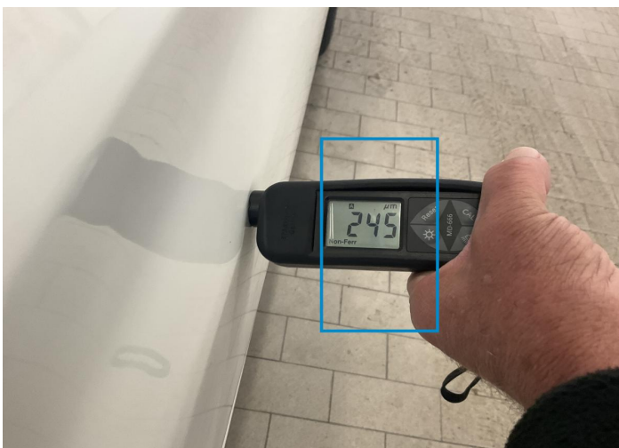
14. Door / Front Right Paint / Poor Previous Repair -
