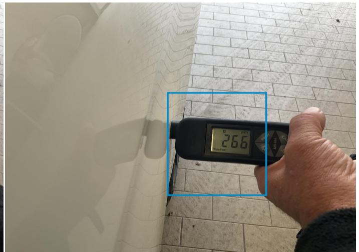
10. Door / Back Left Paint / Poor Previous Repair -
