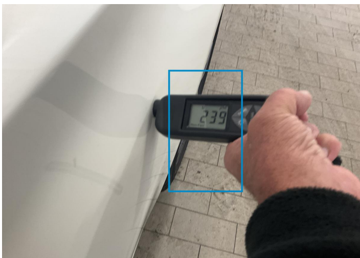
13. Fender / Front Right Paint / Poor Previous Repair -
