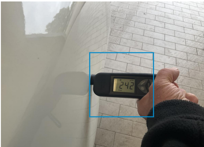
9. Side Panel / Back Left Paint / Poor Previous Repair -
