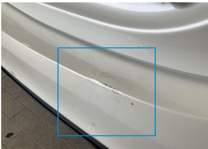
17. Bumper / Back Bodywork / Breakage / Crack -
