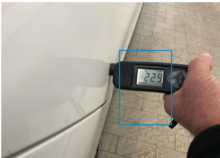
15. Door / Back Right Paint / Poor Previous Repair -
