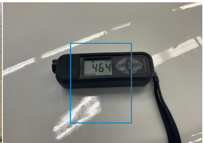
12. Hood Paint / Poor Previous Repair -
