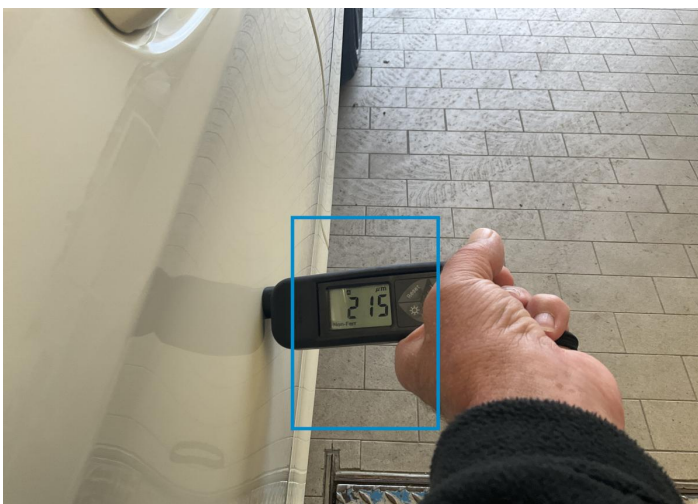
11. Door / Front Left Paint / Poor Previous Repair -
