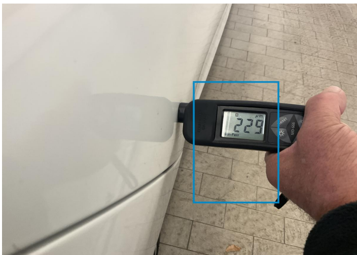
15. Door / Back Right Paint / Poor Previous Repair -
