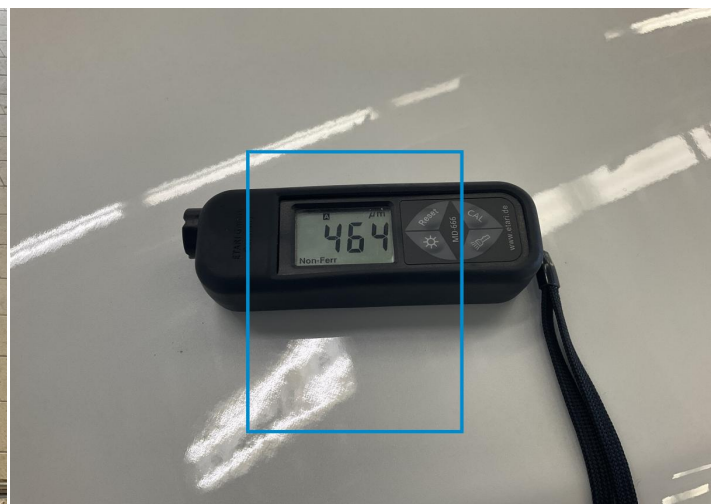
12. Hood Paint / Poor Previous Repair -
