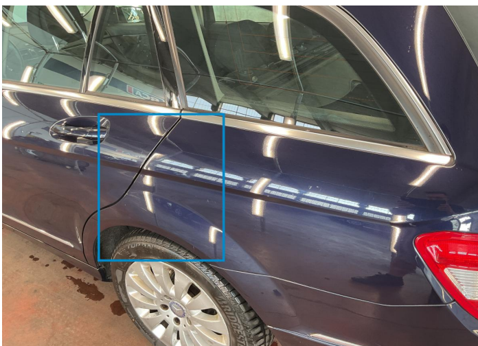
12. Fender / Back Left Bodywork / Dent -
