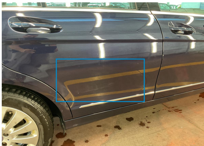
17. Door / Back Right Paint / Scratch / Line -
