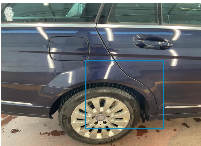
16. Fender / Back Right Bodywork / Dent -
