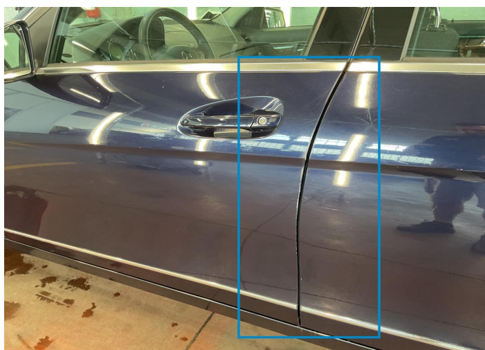
9. Door / Front Left Paint / Scratch / Line -
