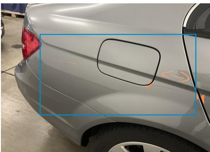
6. Side Panel / Back Right Paint / Scratch / Scuff -
