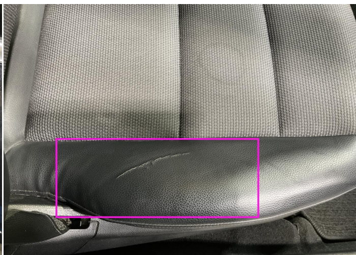
14. Seat / Front Right Interior / Ripped -
