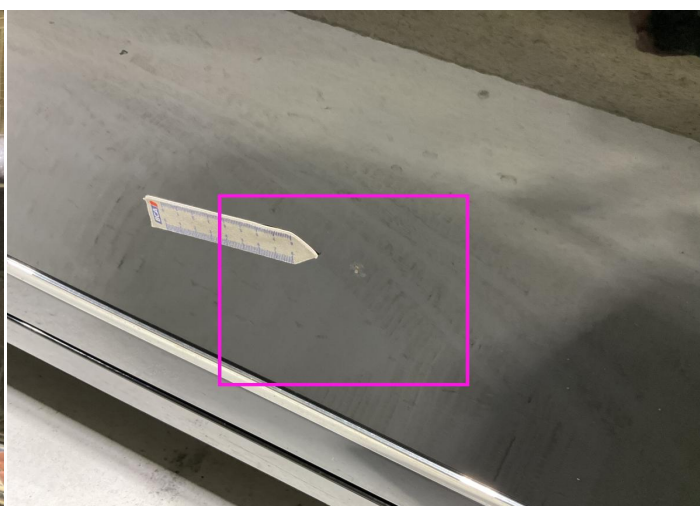
16. Door / Front Right Paint / Scratch / Scuff -
