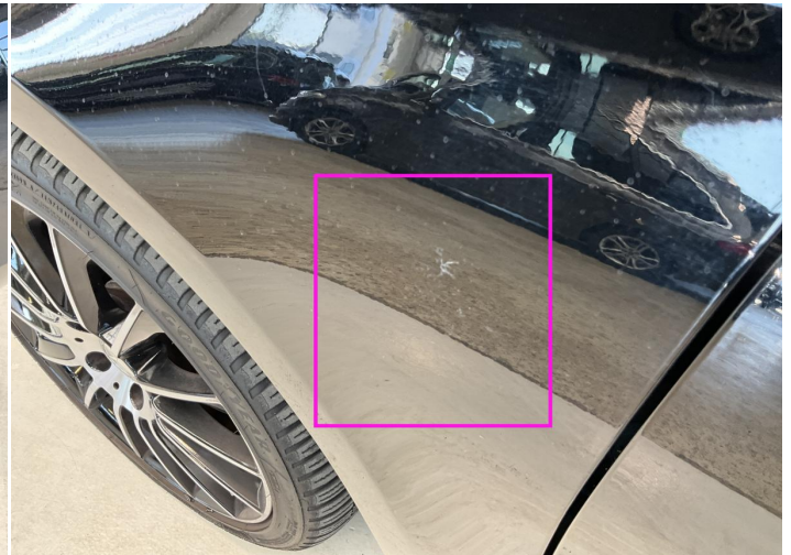
10. Wing Expander / Front Left Paint / Scratch / Scuff -
