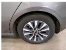
Alloy rim FL polished, Chemical polution, Acceptable
