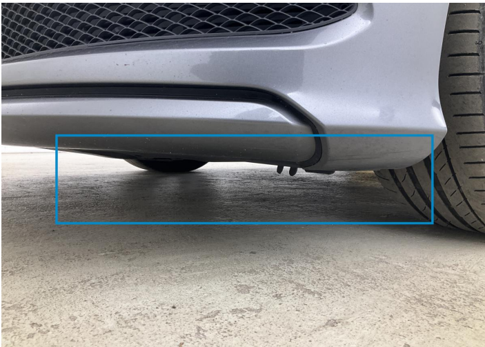
6. Corner Bumper / Front Left Paint / Scratch / Scuff -
