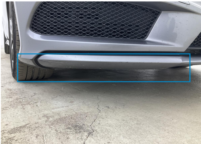
7. Corner Bumper / Front Right Paint / Scratch / Scuff -
