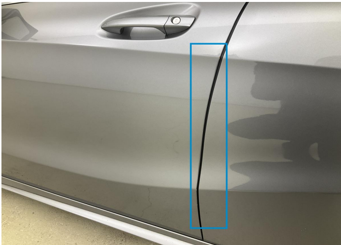
11. Door / Front Left Paint / Scratch / Line -
