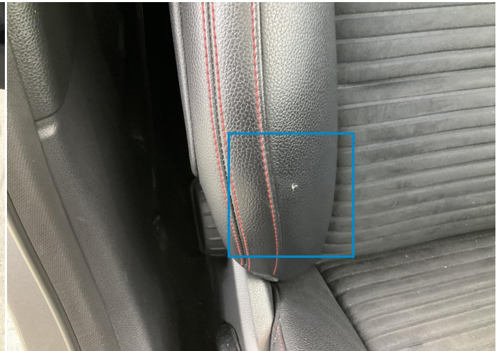
20. Seat / Front Right Interior / Holed -
