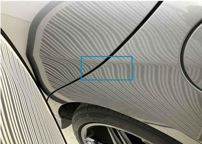
4. Side Panel / Back Left Bodywork / Dent / Dent -
