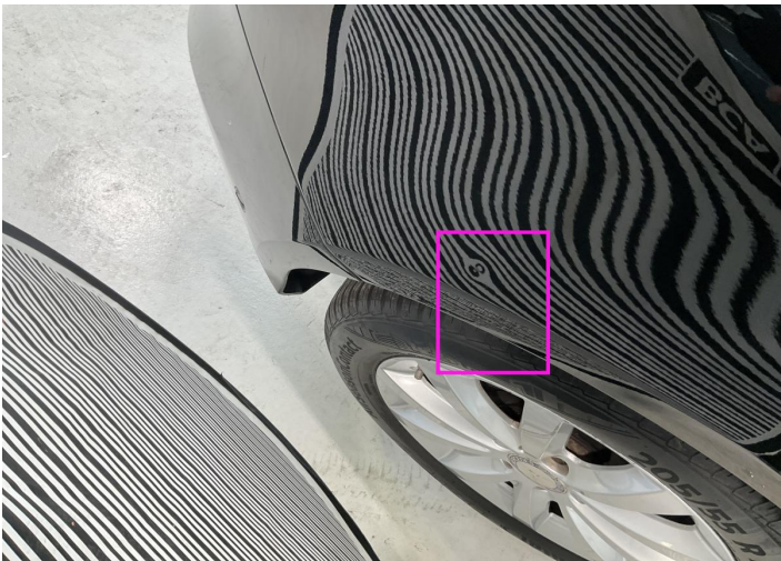
12. Side Panel / Back Right Bodywork / Dent / Dent -
