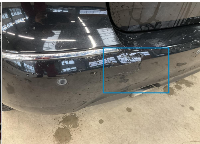
10. Bumper / Back Bodywork / Breakage / Hole -
