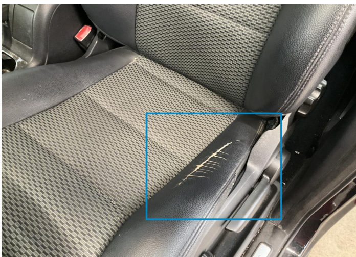
6. Seat / Front Left Interior / Ripped -
