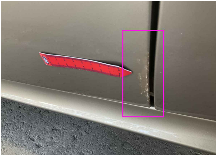
46. Door / Front Left Paint / Poor Previous Repair -
