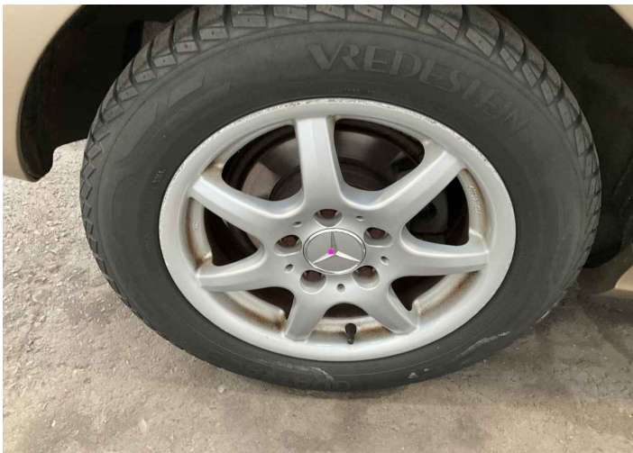
44. Rim / Back Right Out of Bodywork / Scratch -
