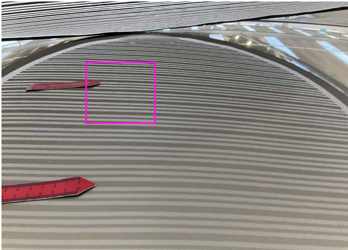
39. Roof Bodywork / Dent / Dent -
