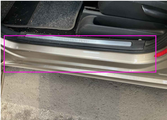
1. Rocker Panel / Center Left Paint / Scratch / Scuff -
