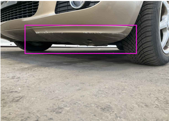
18. Corner Bumper / Front Left Paint / Scratch / Scuff -
