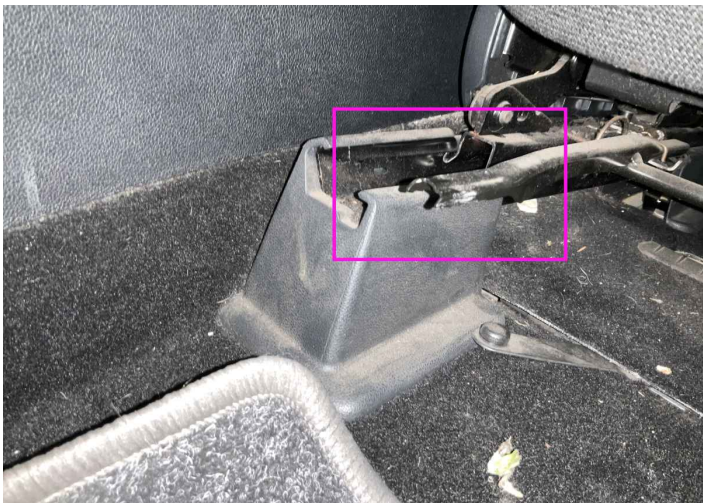
7. Seat / Front Left Interior / Broken -
