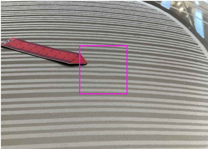
38. Roof Bodywork / Dent / Dent -
