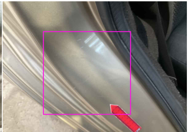
4. Pillar / Back Right Paint / Scratch / Scuff -
