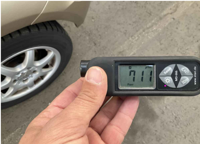
9. Fender / Back Left Paint / Poor Previous Repair -
