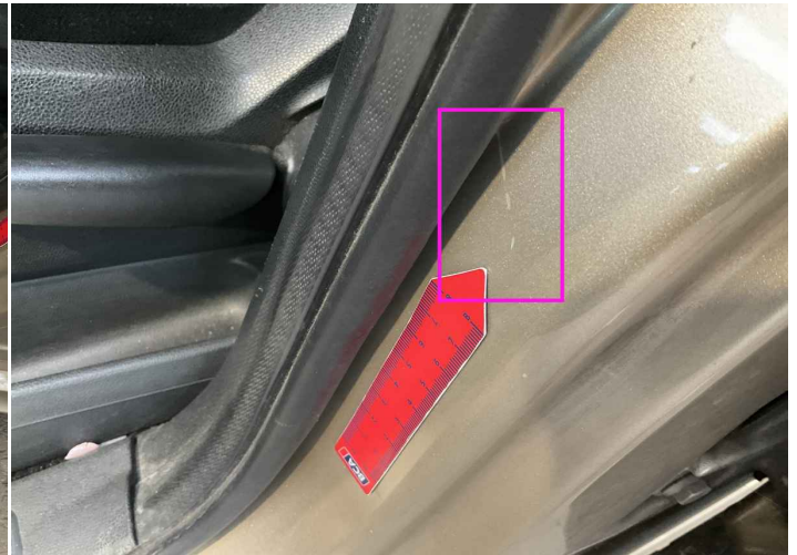
2. B Pillar / Center Left Paint / Scratch / Scuff -
