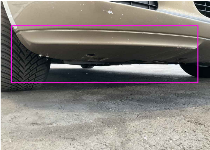
16. Corner Bumper / Front Right Bodywork / Breakage -
