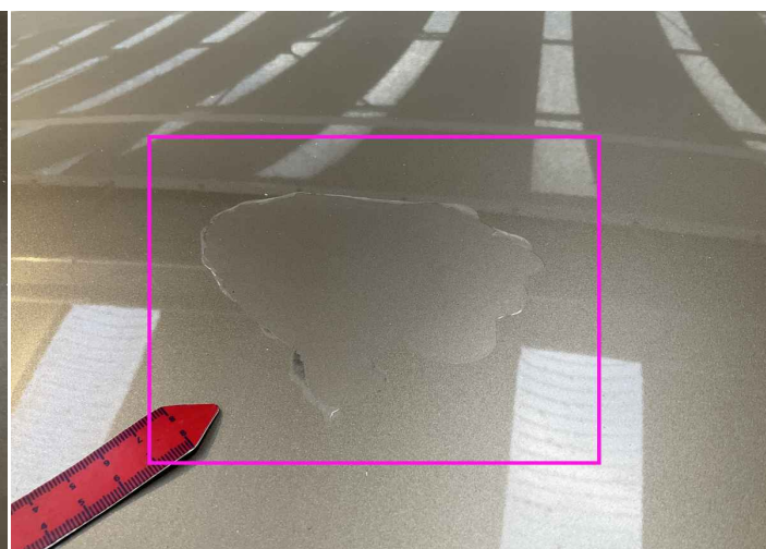
32. Roof Paint / Chipping -
