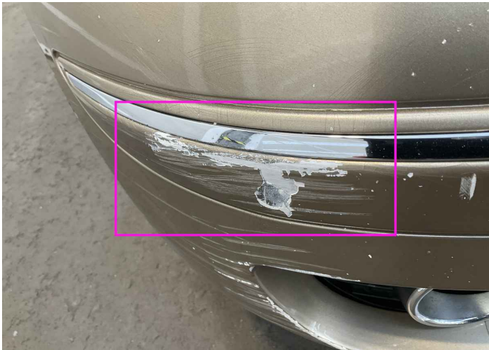
15. Corner Bumper / Front Right Bodywork / Breakage -
