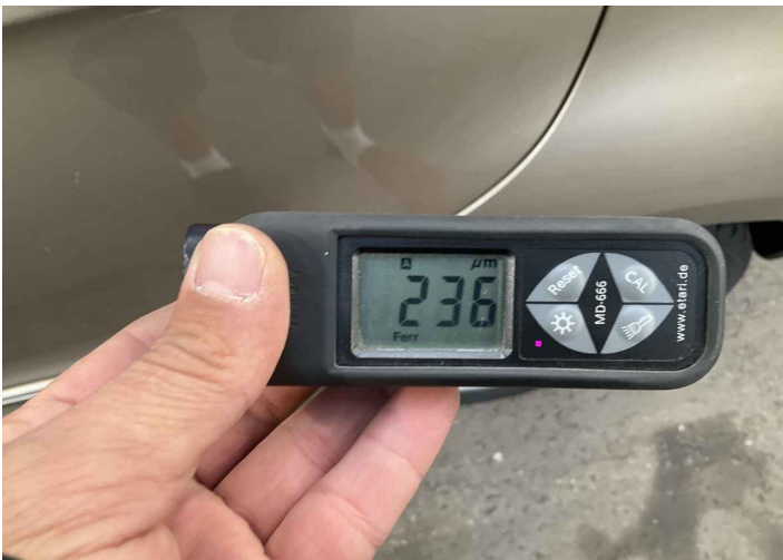
8. Door / Back Left Paint / Poor Previous Repair -
