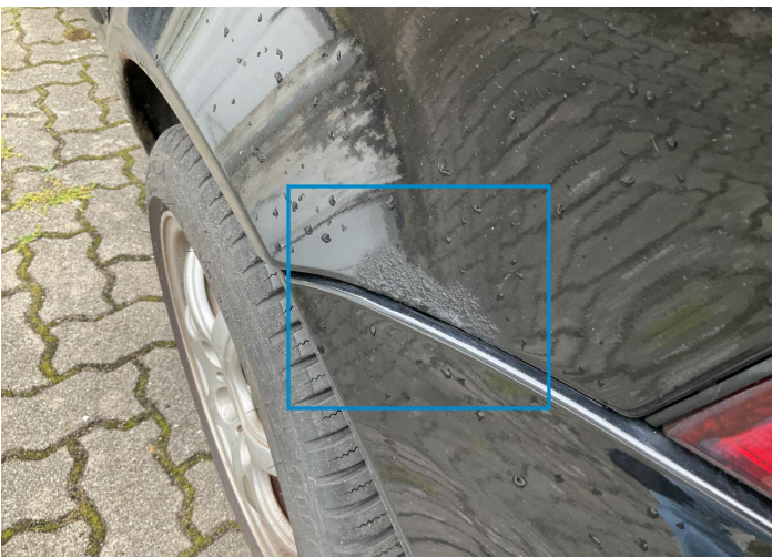
23. Side Panel / Back Left Paint / Corrosion -
