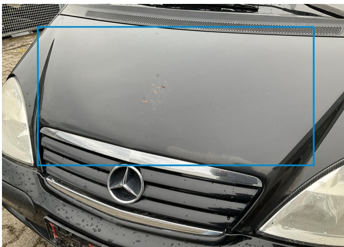
7. Hood Paint / Corrosion -
