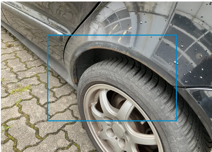
16. Wheel Arch / Back Left Paint / Corrosion -
