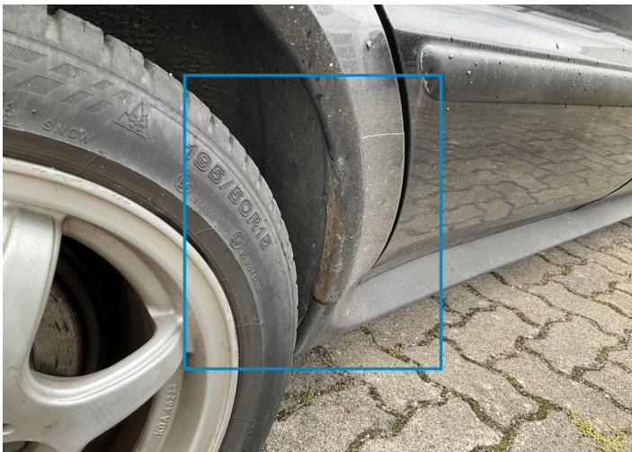
13. Wheel Arch / Back Right Paint / Corrosion -
