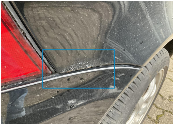
15. Side Panel / Back Right Paint / Corrosion -
