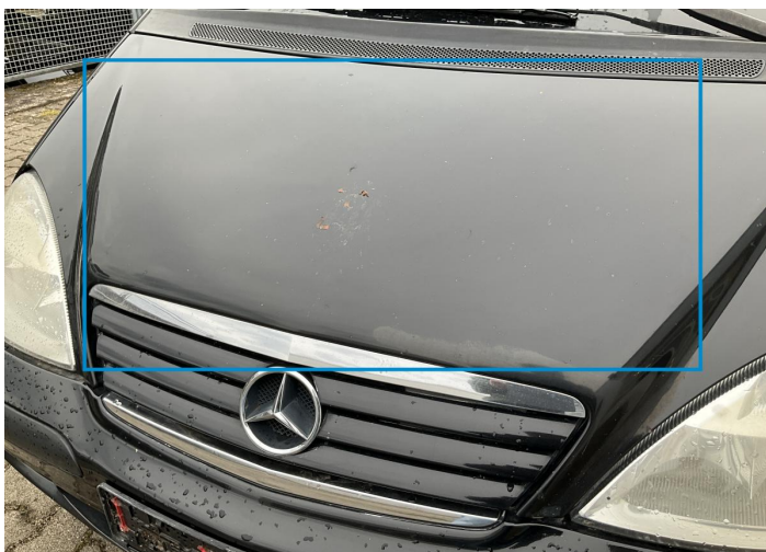
7. Hood Paint / Corrosion -
