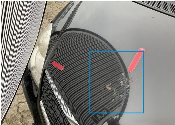
4. Hood Paint / Chemical Damage -
