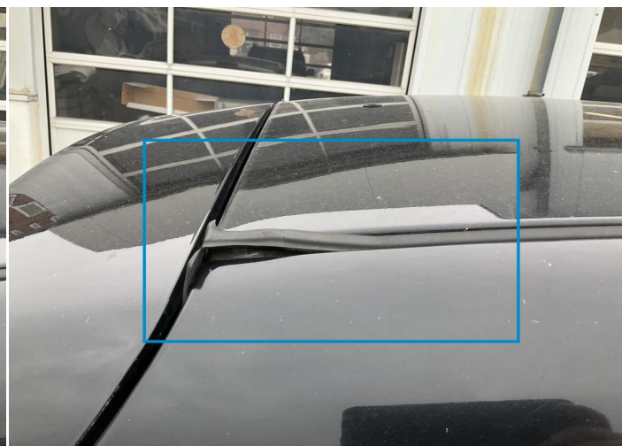
12. Roof Molding / Right Out of Bodywork / Breakage -
