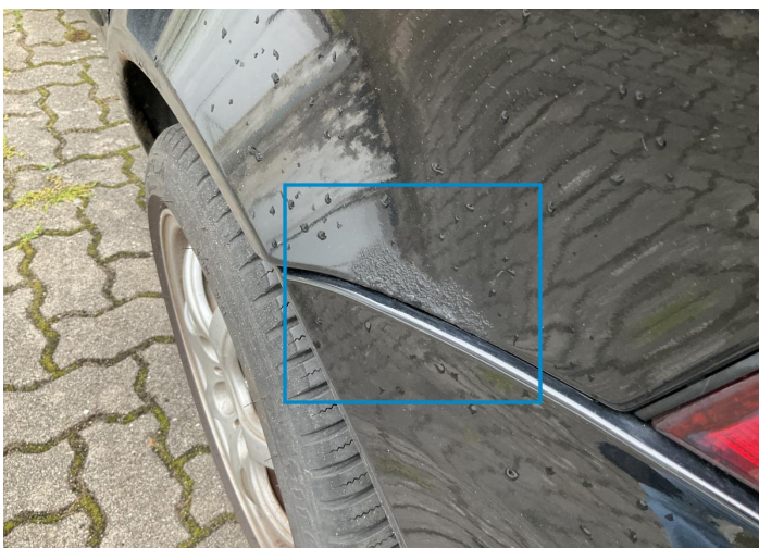
23. Side Panel / Back Left Paint / Corrosion -
