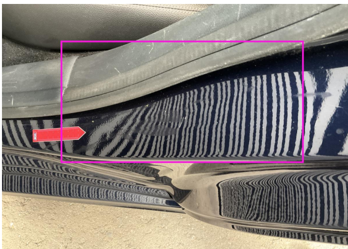
7. Rocker Panel / Center Left Bodywork / Dent / Dent -
