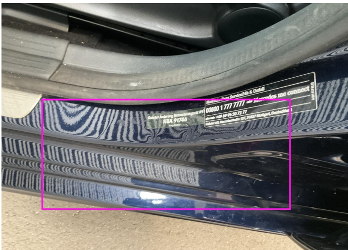
5. Rocker Panel / Center Left Bodywork / Dent / Dent -
