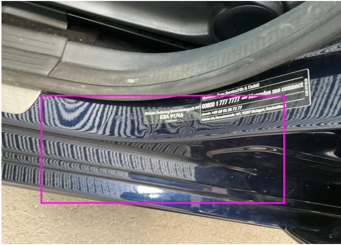
5. Rocker Panel / Center Left Bodywork / Dent / Dent -
