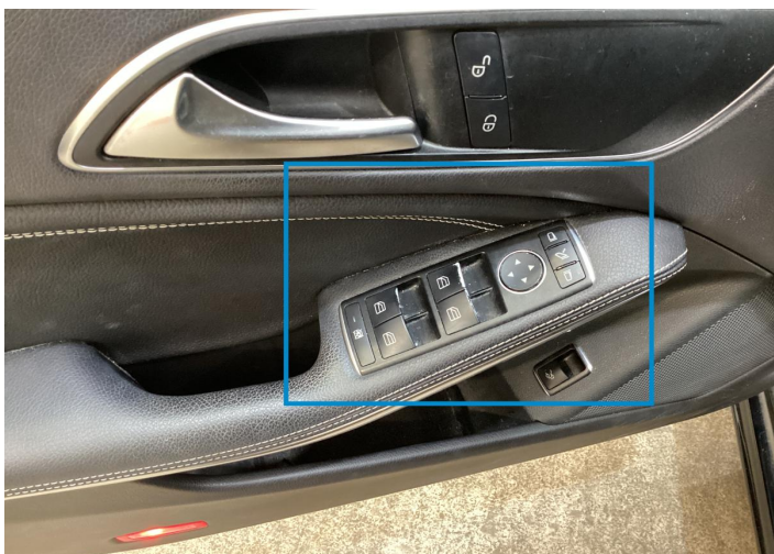
1. Window Switch / Front Left Interior / Worn - out -
