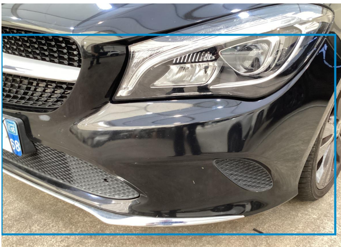
10. Corner Bumper / Front Left Paint / Chipping -
