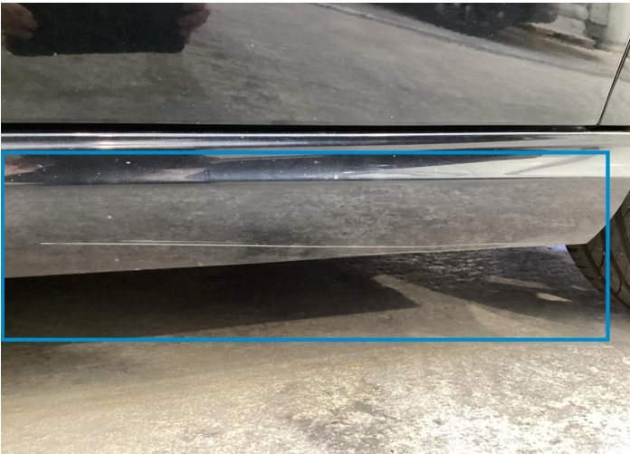
13. Rocker Panel / Center Left Paint / Scratch / Line -
