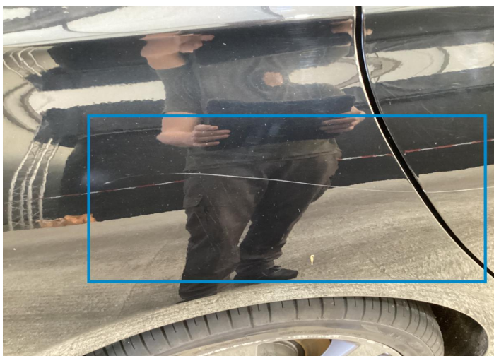
25. Fender / Back Right Paint / Scratch / Line -
