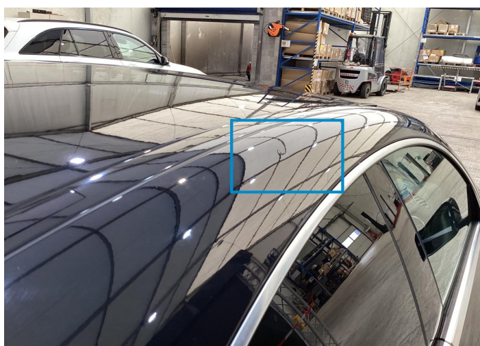
23. Cant Rail / Right Bodywork / Dent / Deformation -
