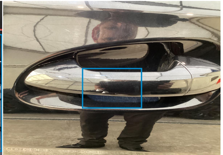
16. Door Handle / Back Left Paint / Scratch / Line -
