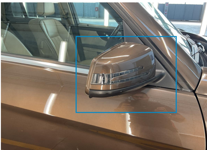
12. Mirror Shell / Front Right Paint / Scratch / Line -
