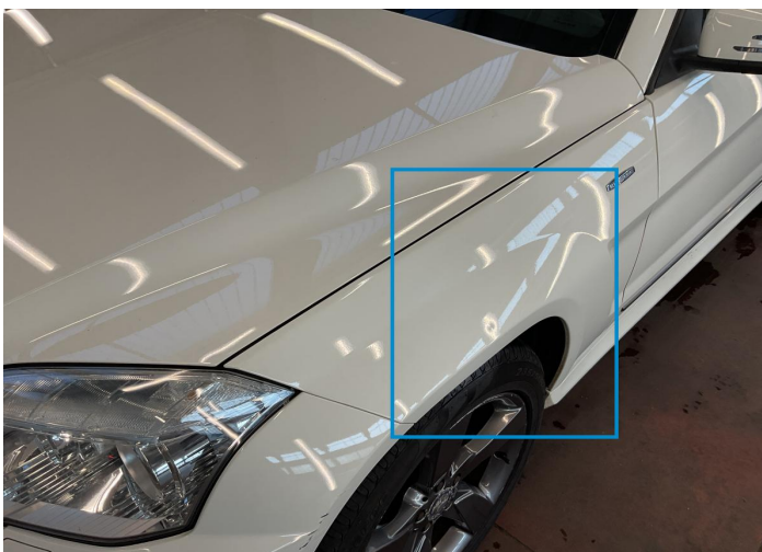
12. Fender / Front Left Bodywork / Dent -
