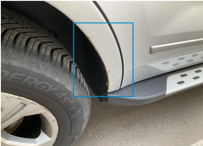
4. Side Panel / Back Right Paint / Corrosion -
