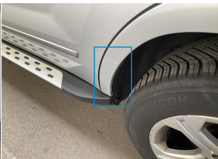
10. Side Panel / Back Left Paint / Corrosion -
