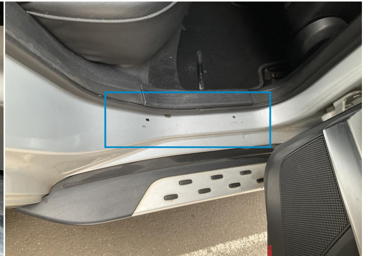
16. Foot Step / Right Missing Part -
