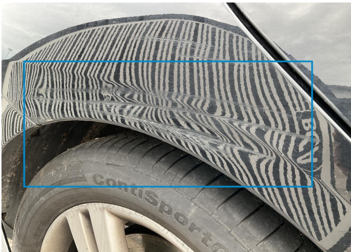
16. Side Panel / Back Right Bodywork / Dent / Dent -
