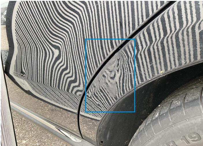
9. Side Panel / Back Left Bodywork / Dent / Dent -
