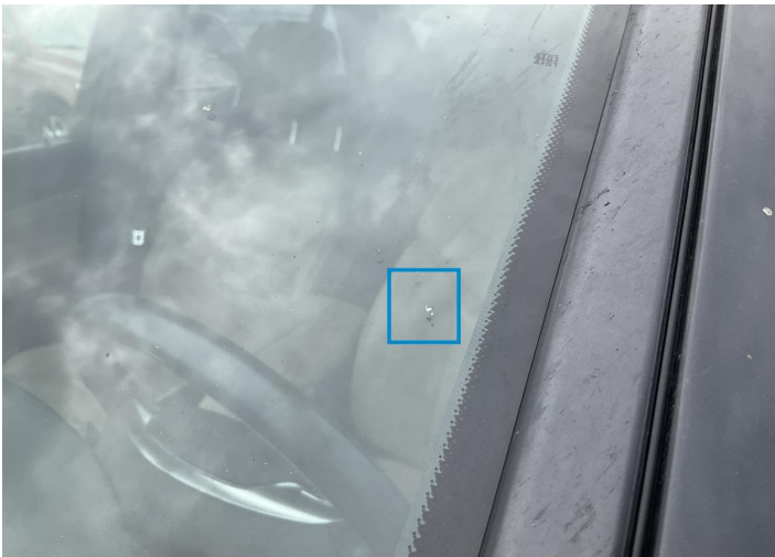
12. Windshield / Front Glass Break / Impact -
