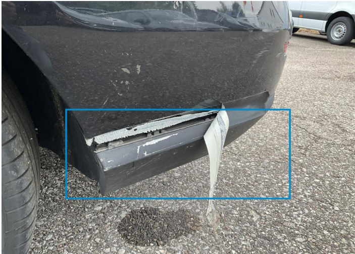
5. Bumper / Back Bodywork / Breakage / Crack -
