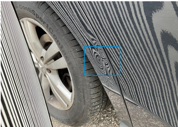
15. Side Panel / Back Right Bodywork / Dent / Dent -
