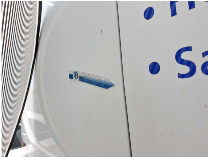
Damage 5: Body: Body (Flugrost) - Paint defect - Conditioning
