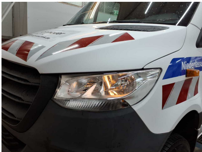
Damage 2: Headlight: Headlight - left side (Abblendlicht) - Defective - Replace
