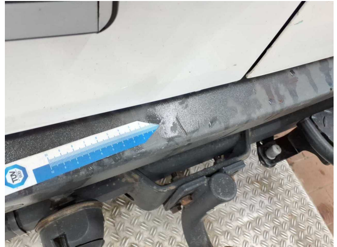
Wear and tear 4: Rear bumper: Rear bumper (unpainted) (Verladebereich / Einstieg) - Scratch(es) - No deduction
