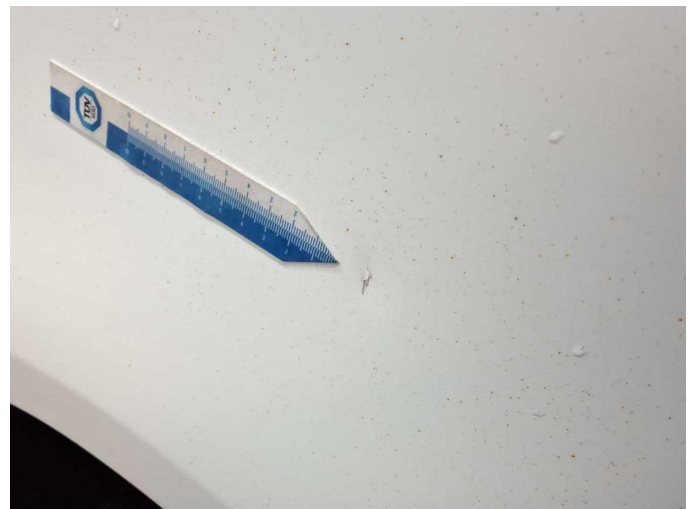
Damage 5: Body: Body (Flugrost) - Paint defect - Conditioning
