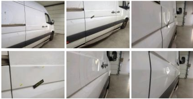
Wing FR, Dent(s), Repair and paint (complete)
