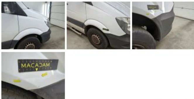
Mirror side repeater R, Scratch(es), Replace
