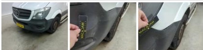
Bumper F, Dent(s) and scratch(es), Replace
