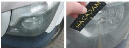
Headlight R, Crack, Replace
