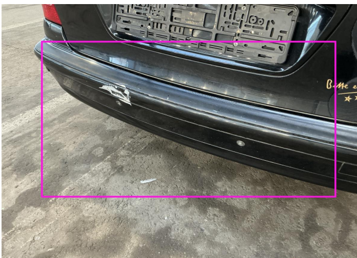
20. Bumper / Back Bodywork / Breakage / Crack -
