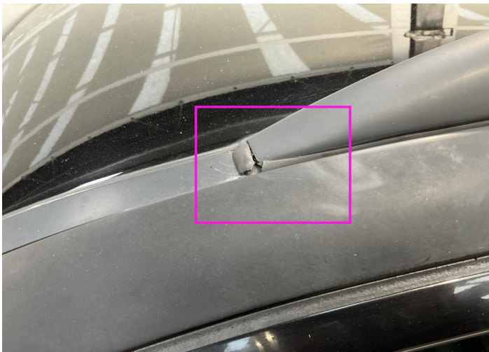
1. Roof Rack / Left Out of Bodywork / Breakage -
