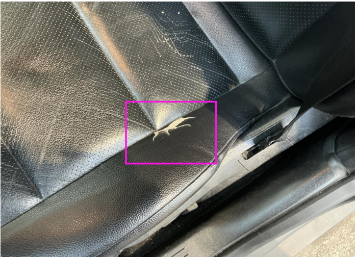
33. Seat / Front Left Interior / Ripped -
