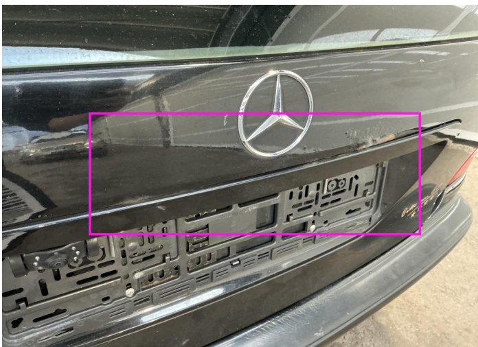
22. Tailgate Paint / Corrosion -
