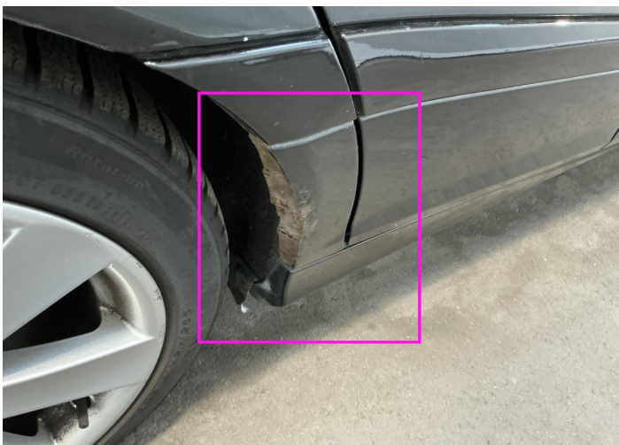
16. Fender / Back Right Paint / Corrosion -
