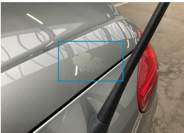
24. Tailgate Paint / Poor Previous Repair -
