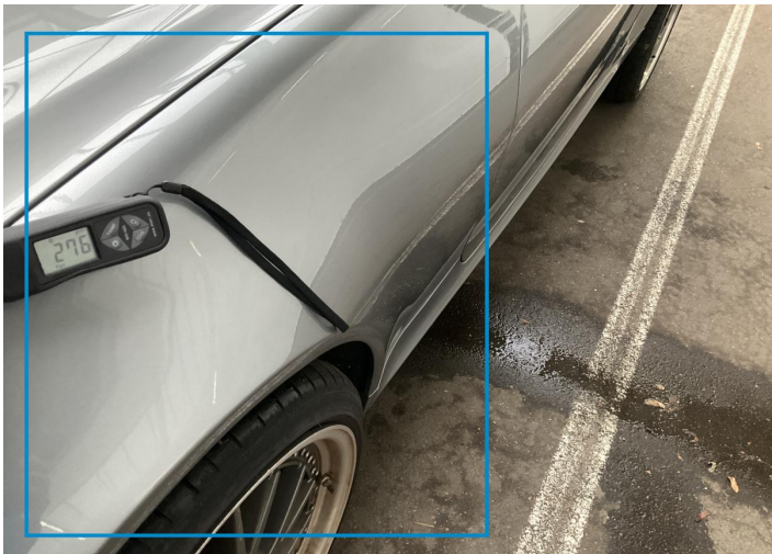
12. Fender / Front Left Paint / Poor Previous Repair -
