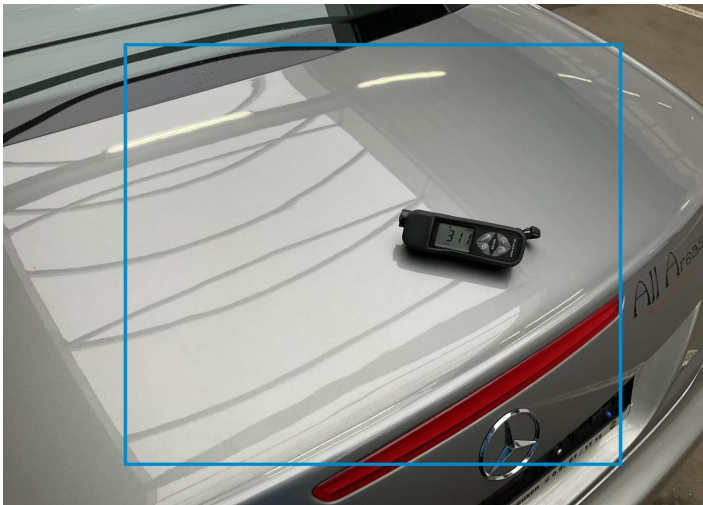
11. Tailgate Paint / Poor Previous Repair -
