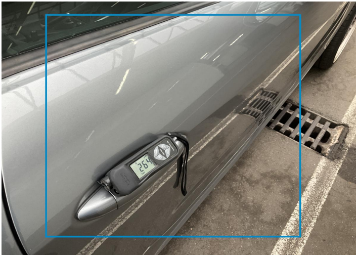
10. Door / Front Right Paint / Poor Previous Repair -
