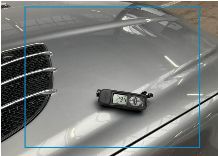
8. Hood Paint / Poor Previous Repair -
