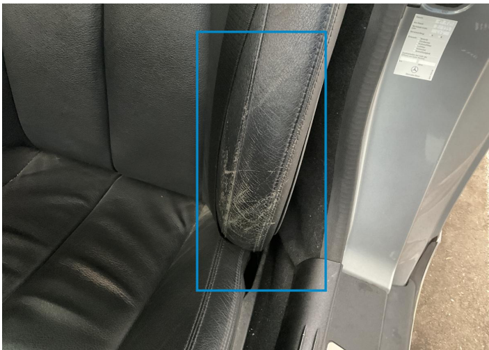
1. Seat / Front Left Interior / Worn - out -
